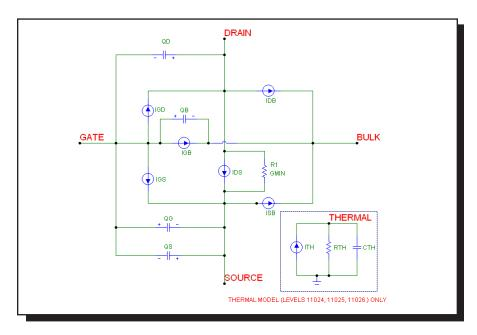
Figure 25-21 Electrical model of Philips Model 11
