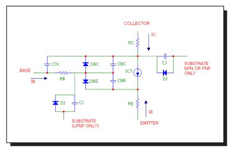
Figure 25-1 Bipolar transistor model
