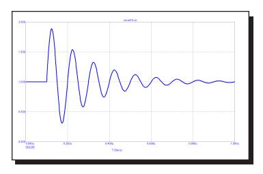
Figure 25-13 Waveform for "SIN 1 1 10Meg 100n 5E6"
