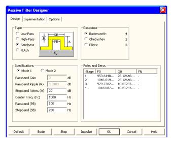
Figure 32-11 The passive filter design panel
