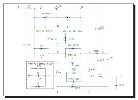
Figure 25-2 Mextram bipolar transistor model
