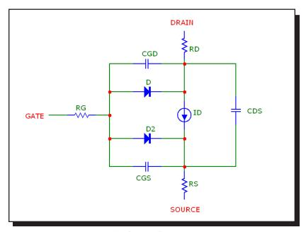
Figure 25-8 The GaAsFET model
