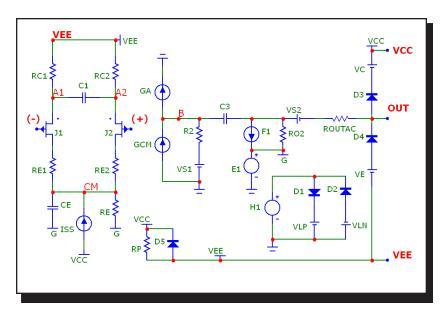
Figure 25-31 The level 3 opamp model with JFET inputs
