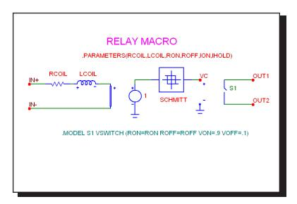
Figure 24-39 RELAY1 macro circuit
