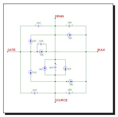
Figure 25-25 PSP model equivalent circuit
