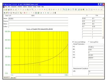
Figure 30-4 The Vce vs. Ic Plot
