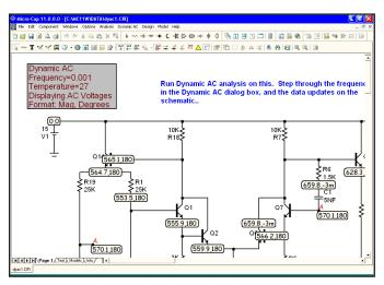
Figure 9-3 AC voltages in mag, phase (degrees)
