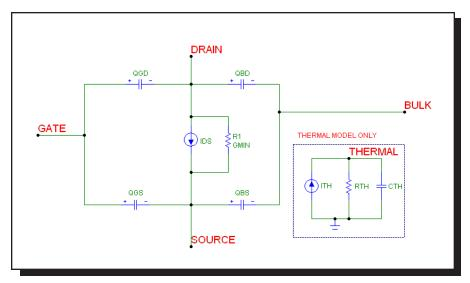
Figure 25-23 Philips Model 31 equivalent circuit
