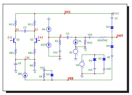
Figure 25-29 The level 3 opamp model with NPN inputs
