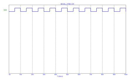
Figure 26-5 Stimulus waveform for example 3
