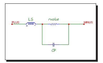
Figure 25-33 Resistor model
