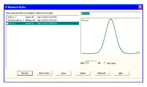
Figure 15-2 The Waveform Buffer dialog box
