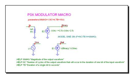
Figure 24-35 PSK macro circuit
