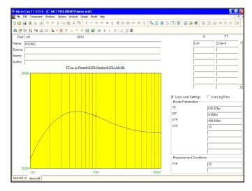
Figure 30-8 The FT vs. Ic Plot
