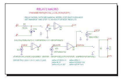
Figure 24-40 RELAY2 macro circuit
