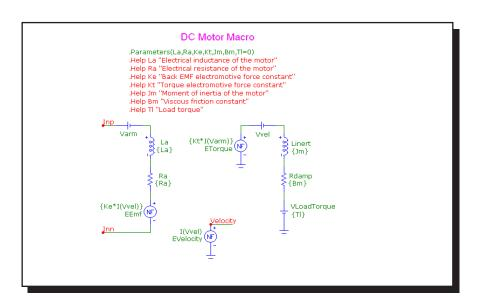
Figure 24-11 DC Motor macro circuit
