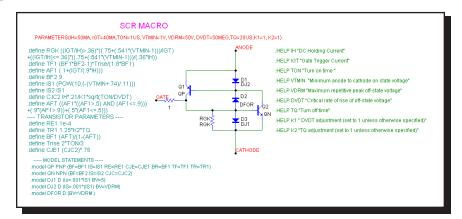
Figure 24-44 SCR macro circuit
