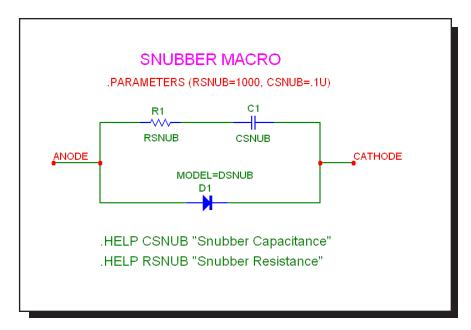
Figure 24-46 SNUBBER macro circuit
