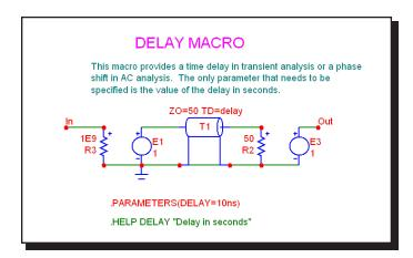
Figure 24-12 DELAY macro circuit
