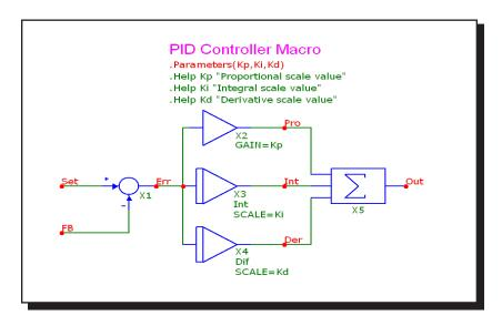
Figure 24-33 PID Controller macro circuit
