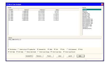
Figure 20-05 The Worst Case dialog box for the BP filter
