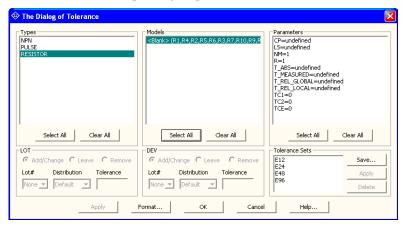
Figure 19-4 The Tolerance dialog box
