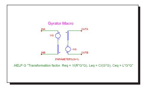
Figure 24-20 GYRATOR macro circuit
