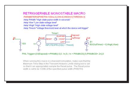
Figure 24-27 MONOSTABLE RT macro circuit
