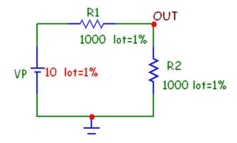
Figure 20-1 The WC\_DC\_OP0 circuit, a simple voltage divider
