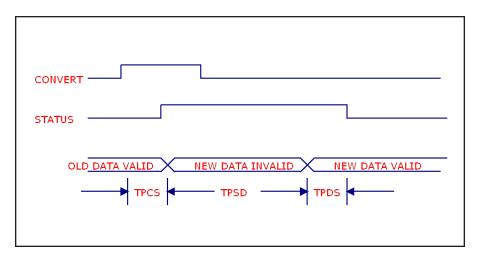
Figure 26-2 ADC timing diagram
