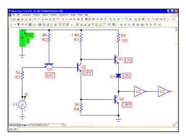
Figure 10-6 Display of device conditions
