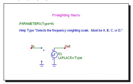
Figure 24-19 FWeighting macro circuit
