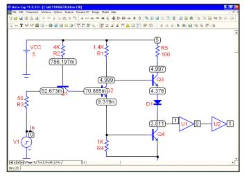
Figure 10-2 Display of initial node voltages
