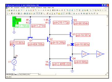
Figure 10-5 Display of device power terms
