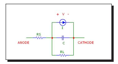
Figure 25-7 Diode model
