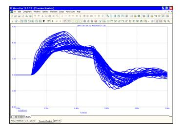
Figure 21-6 Stepping both C1 and R1
