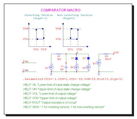
Figure 24-8 COMPARATOR macro equivalent circuit
