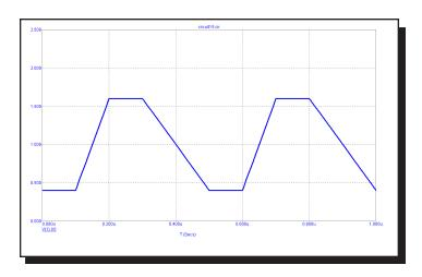
Figure 25-11 Waveform for "PULSE .4 1.6 .1u .1u .2u .1u .5u"
