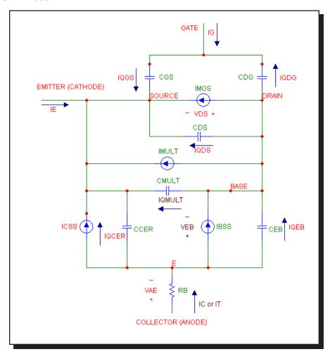
Figure 25-9 The IGBT model
