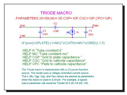
Figure 24-53 TRIODE macro circuit
