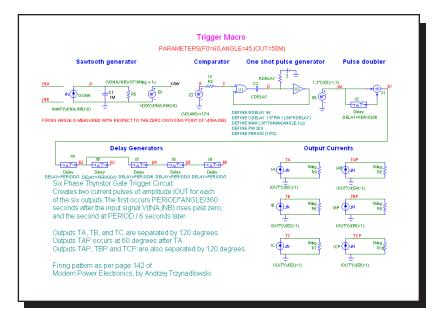
Figure 24-52 TRIGGER6 macro circuit
