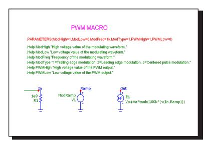
Figure 24-37 PWM Controller macro circuit
