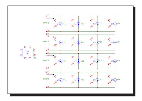
Figure 25-26 Four port equivalent circuit
