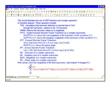
Figure 34-1 The FFT1 circuit
