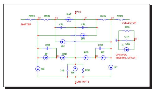
Figure 25-3 Modella lateral PNP transistor model
