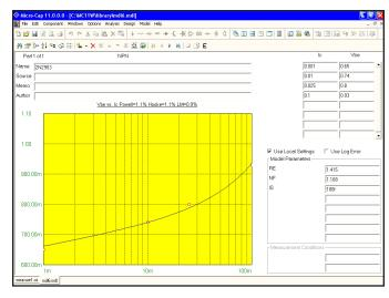
Figure 30-2 The Vbe vs. Ic plot
