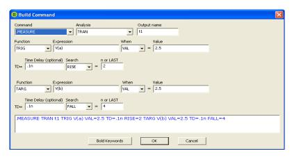
Figure 2-23 . Measure command with TRIG and TARG
