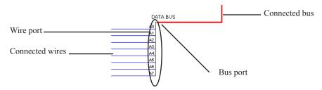
Figure 2-4 Typical bus connector
