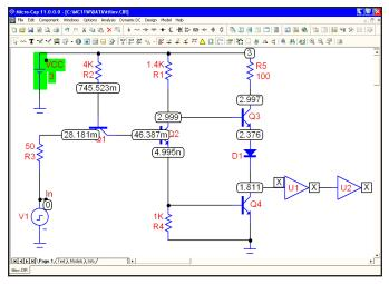
Figure 10-3 Display of voltages at the switching point
