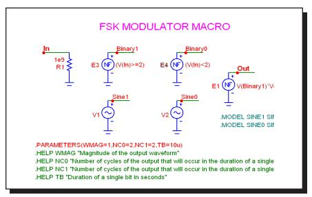
Figure 24-18 FSK macro circuit
