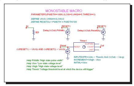
Figure 24-27 MONOSTABLE macro circuit
