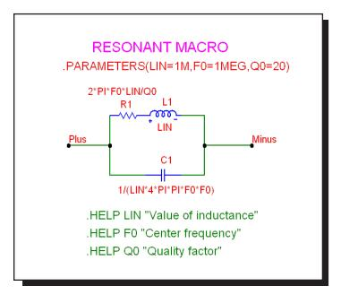
Figure 24-41 RESONANT macro circuit
