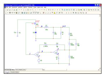
Figure 35-5 SMPS Buck Converter
