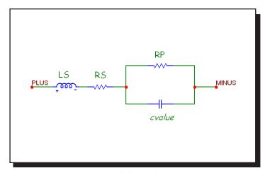
Figure 25-4 Capacitor model
