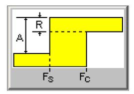
Figure 32-8 High pass filter specifications
