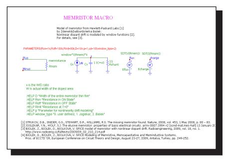
Figure 24-25 Memristor macro circuit
