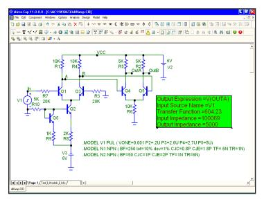
Figure 11-3 The annotated schematic
