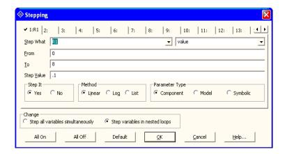
Figure 23-3 R(R1) is stepped from 0 to 8
