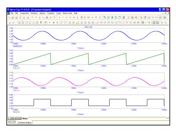
Figure 35-6 Buck converter waveforms
