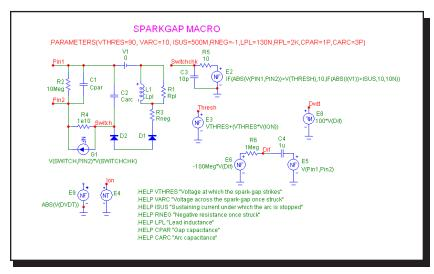
Figure 24-47 SPARKGAP macro circuit
