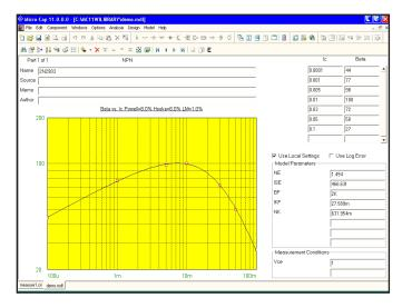
Figure 30-3 The Beta vs. Ic Plot
