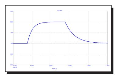
Figure 25-10 Waveform for "EXP 1 2 150n 50n 550n 100n"
