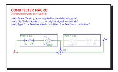
Figure 24-6 Comb Filter macro circuit
