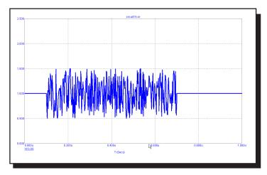
Figure 25-15 NOISE Waveform for "DC 1 AC 1 0 NOISE 2N 1 100N 700N 1"
