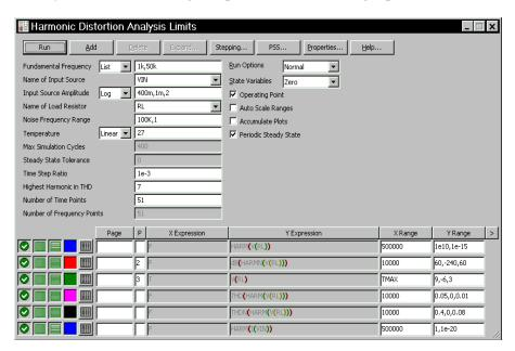
Figure 13-1 Harmonic Distortion Analysis Limits dialog box
