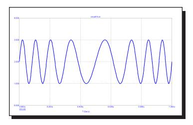
Figure 25-12 Waveform for "SFFM 2 1 8Meg 4 1Meg"
