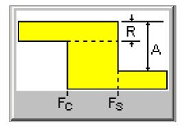
Figure 32-7 Low pass filter specifications
