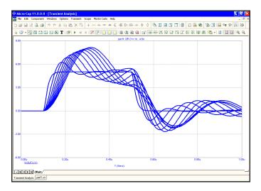
Figure 21-2 The transient analysis run
