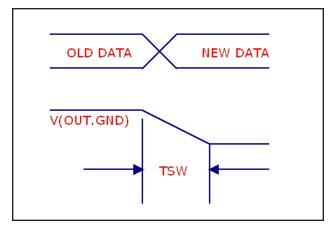
Figure 26-3 DAC timing diagram
