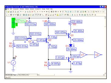
Figure 10-4 Display of device currents
