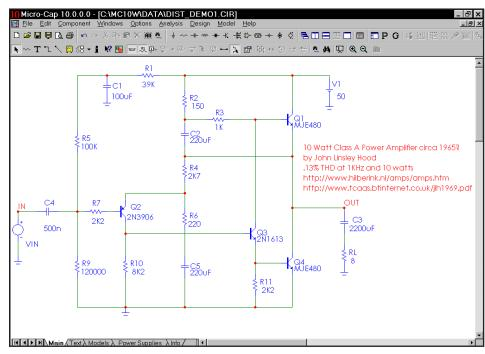
Figure 13-2 Harmonic Distortion sample circuit
