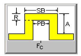
Figure 32-9 Bandpass filter specifications
