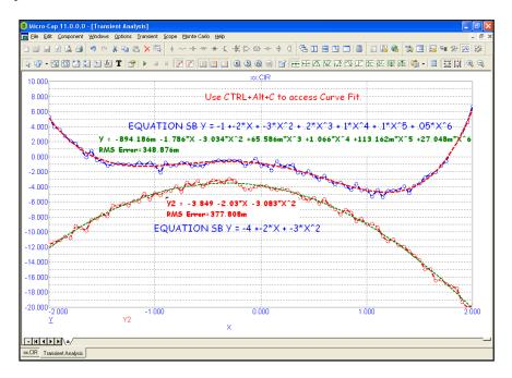
Figure 15-4 Transient plot with two curve fits
