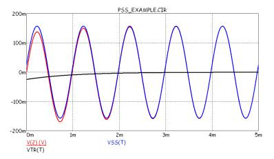
Figure 35-2 Steady state, transient, and total waveforms
