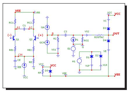
Figure 25-30 The level 3 opamp model with PNP inputs
