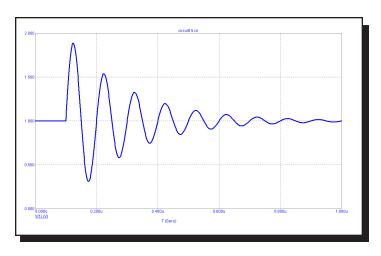
Figure 22-13 Waveform for "SIN 1 1 10Meg 100n 5E6"
