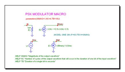
Figure 21-35 PSK macro circuit
