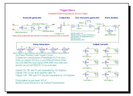
Figure 21-52 TRIGGER6 macro circuit
