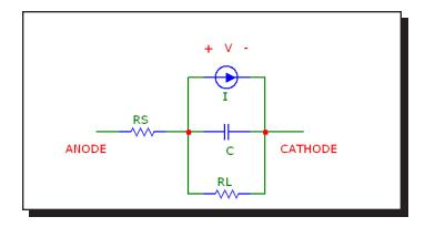
Figure 22-7 Diode model
