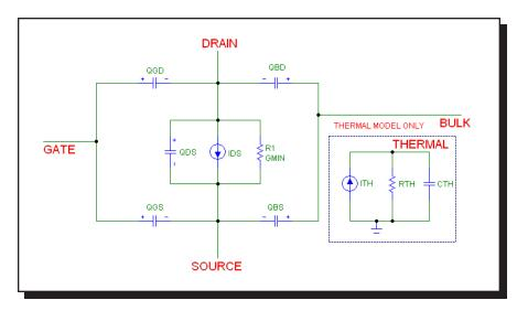
Figure 22-24 Philips Model 40 equivalent circuit
