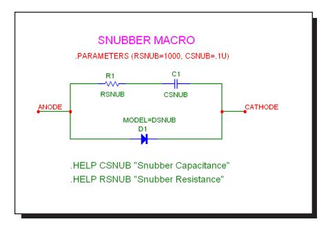
Figure 21-46 SNUBBER macro circuit
