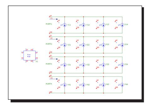
Figure 22-26 Four port equivalent circuit
