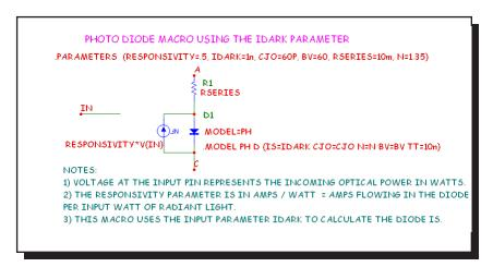
Figure 21-31 PHOTODIODE macro circuit
