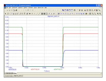
**Figure 23-11 Transient Output Using Different Power Supplies**
