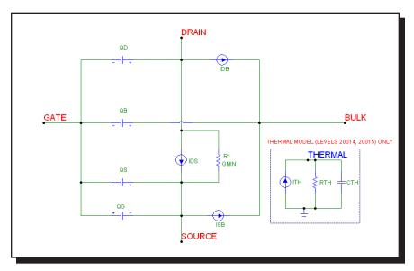
Figure 22-22 Philips Model 20 equivalent circuit
