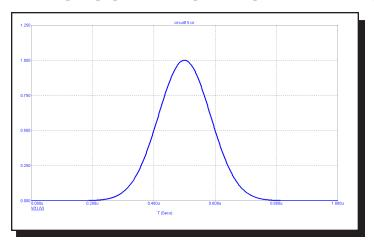
Figure 22-16 GAUSSIAN Waveform for "DC 0 AC 1 0 GAUSSIAN 1 500N 200N 1U"
