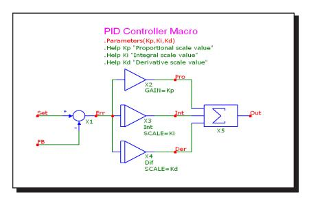
Figure 21-33 PID Controller macro circuit
