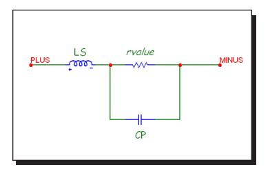
Figure 22-33 Resistor model
