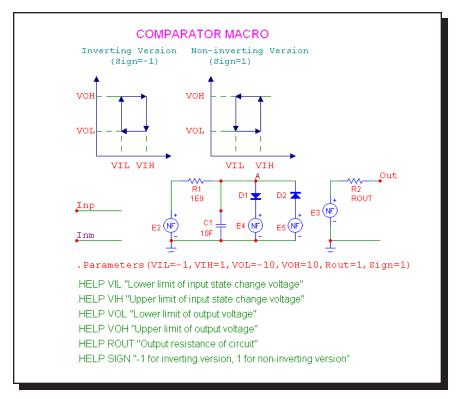
Figure 21-8 COMPARATOR macro equivalent circuit
