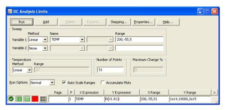
Figure 27-10 DC Analysis Limits for the Steinhart Circuit
