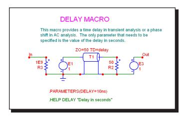
Figure 21-12 DELAY macro circuit
