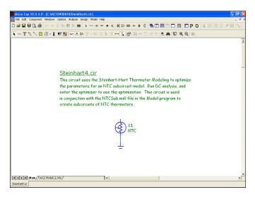
Figure 27-9 NTC Thermistor Optimization Test Circuit
