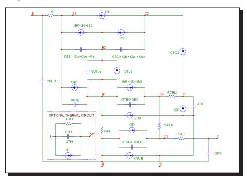
Figure 22-2 Mextram bipolar transistor model
