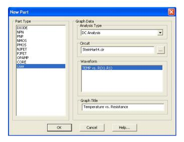
Figure 27-11 New Part Dialog Box Settings for the NTC Subcircuit
