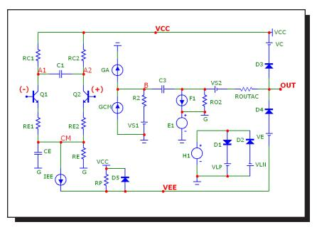
Figure 22-29 The level 3 opamp model with NPN inputs
