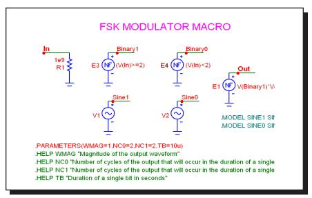
Figure 21-18 FSK macro circuit
