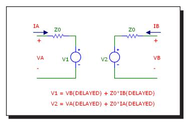
Figure 22-35 Transmission line model
