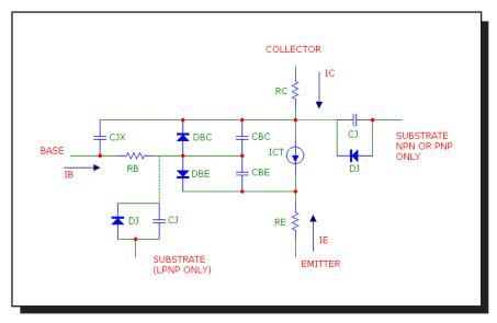
Figure 22-1 Bipolar transistor model
