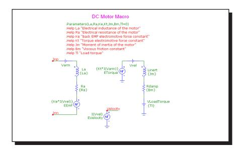
Figure 21-11 DC Motor macro circuit
