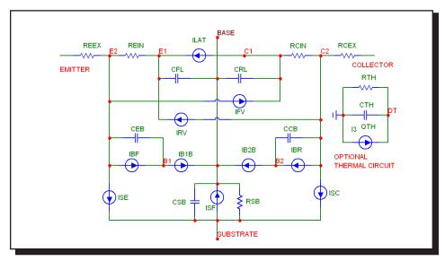
Figure 22-3 Modella lateral PNP transistor model
