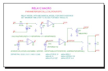
Figure 21-40 RELAY2 macro circuit
