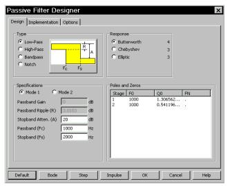
Figure 29-11 The passive filter design panel
