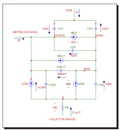
Figure 22-9 The IGBT model
