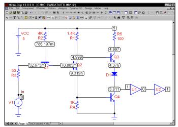
Figure 10-2 Display of initial node voltages
