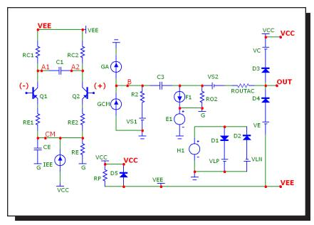
Figure 22-30 The level 3 opamp model with PNP inputs
