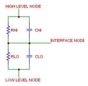
Figure 23-8 N device equivalent circuit
