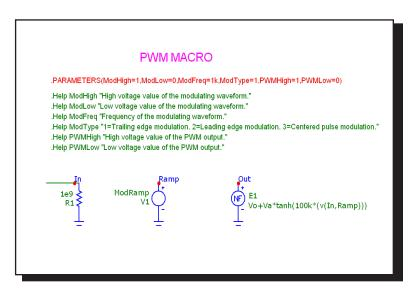
Figure 21-37 PWM Controller macro circuit
