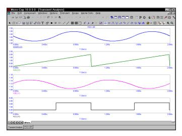
Figure 32-6 SMPS Buck converter waveforms
