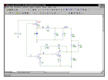
Figure 32-5 SMPS Buck Converter
