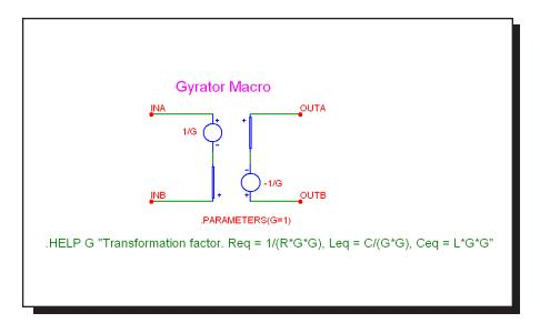
Figure 21-20 GYRATOR macro circuit
