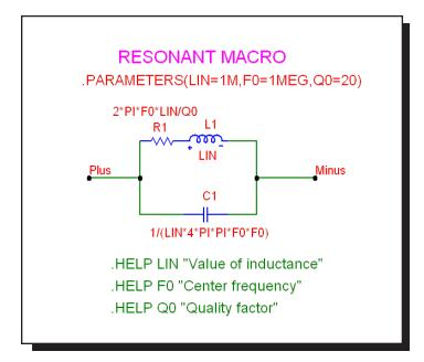
Figure 21-41 RESONANT macro circuit
