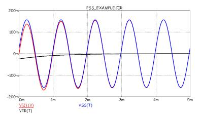
Figure 32-2 Steady state, transient, and total waveforms
