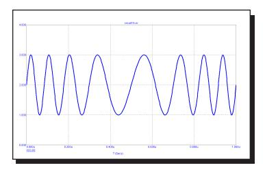
Figure 22-12 Waveform for "SFFM 2 1 8Meg 4 1Meg"
