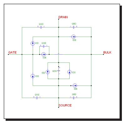
Figure 22-25 PSP model equivalent circuit
