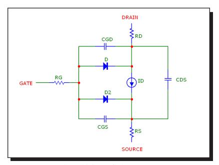
Figure 22-8 The GaAsFET model
