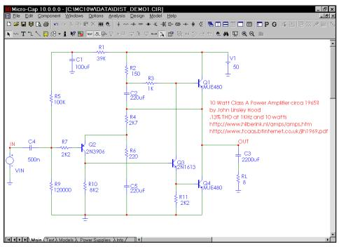
Figure 13-2 Harmonic Distortion sample circuit
