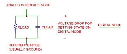
Figure 23-9 O device equivalent circuit
