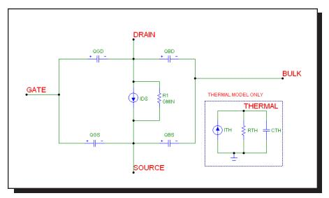
Figure 22-23 Philips Model 31 equivalent circuit
