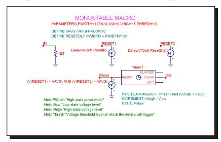
Figure 21-27 MONOSTABLE macro circuit
