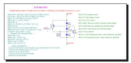
Figure 21-44 SCR macro circuit
