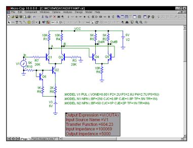
Figure 11-3 The annotated schematic
