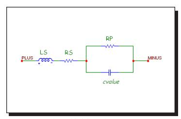
Figure 22-4 Capacitor model
