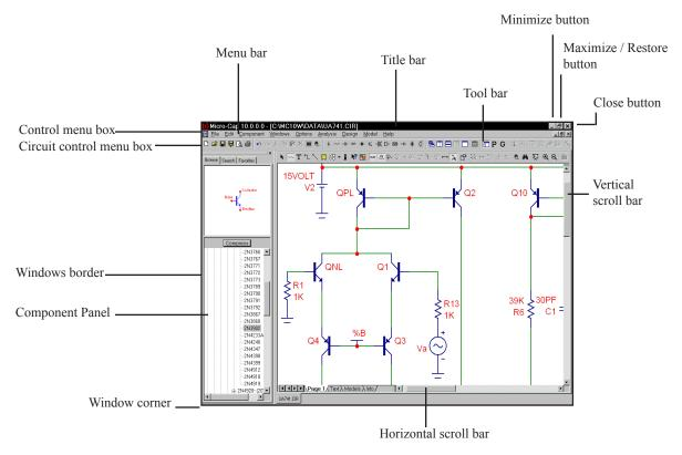
Figure 1-1 The parts of a window
