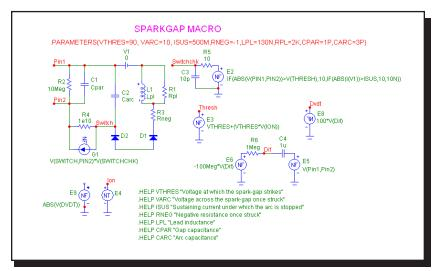
Figure 21-47 SPARKGAP macro circuit
