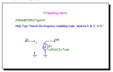
Figure 21-19 FWeighting macro circuit
