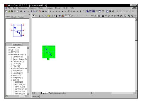
Figure 2-17 The Component panel
