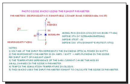
Figure 21-32 PHOTODIODE\_R macro circuit
