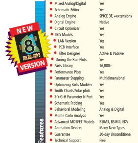
It's all here—in Micro-Cap 8.0, the fast, mixed-mode analog/digital SPICE-based simulator that incorporates an intuitive eighth-generation user interface, a 16,000 part library, a built-in circuit optimizer and the latest device models.
