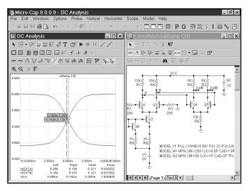
Figure 8-10 Using the cursors to find the peak gain
