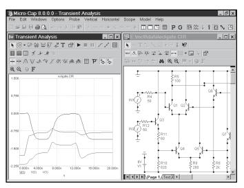
Figure 8-1 Probing node voltages
