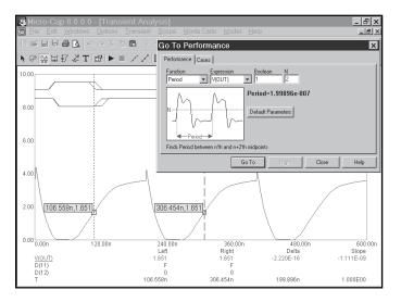
Figure 7-20 Measuring the pulse period
