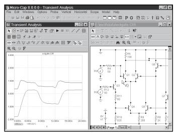
Figure 8-2 Probing lead-to-lead voltages
