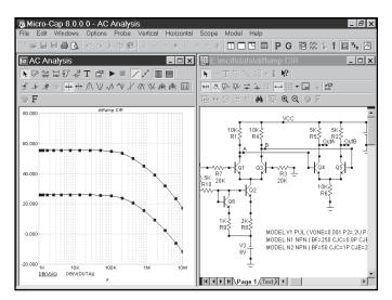
Figure 8-6 Reading AC gains using the Cursor mode
