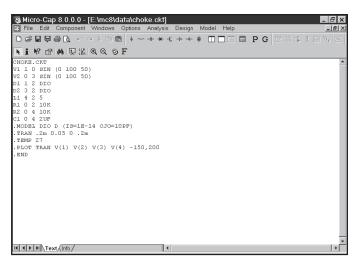
Figure 3-21 The sample SPICE circuit
