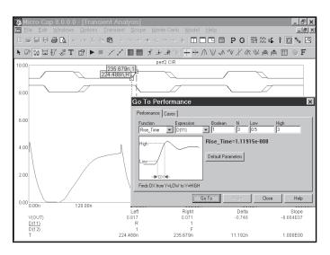
Figure 7-24 Measuring digital rise times
