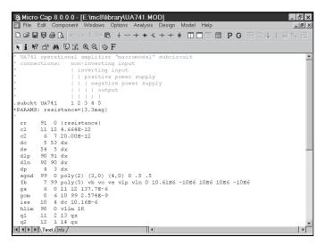
Figure 12-1 The UA741.MOD subcircuit
