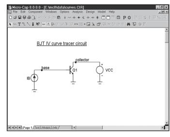
Figure 2-15 The IVBJT circuit
