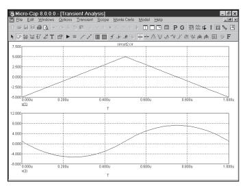
Figure 11-5 Transient analysis of the circuit
