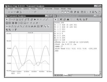
Figure 8-11 Probing SPICE circuits
