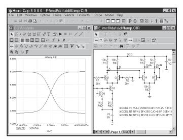
Figure 8-9 DC transfer function plot
