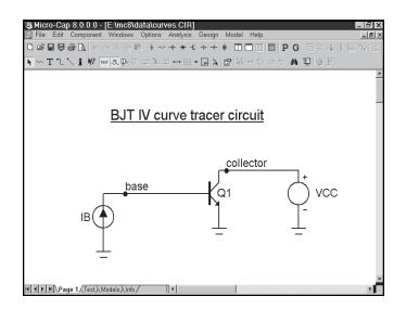
Figure 6-1 The CURVES circuit
