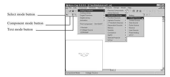
Figure 3-1 Selecting a part from the Component menu
