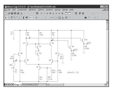
Figure 2-10 The RCA3040 circuit
