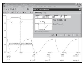
Figure 7-21 Measuring the pulse width
