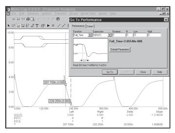
Figure 7-19 Measuring fall time
