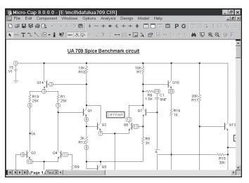
Figure 3-17 The UA709 circuit
