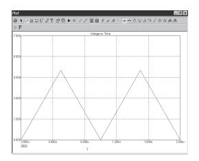
Figure 3-4 Characteristic plot of the source with TF=500n
