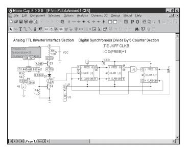
Figure 2-6 Operating point node voltages and states
