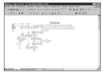
Figure 10-5 Display of device power terms
