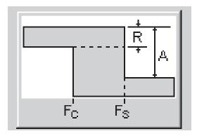
Figure 29-7 Low pass filter specifications
