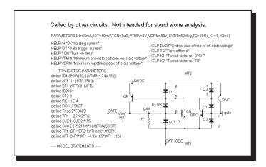
Figure 21-34 TRIAC macro equivalent circuit
