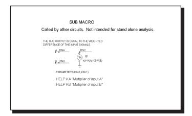
Figure 21-31 SUB macro equivalent circuit
