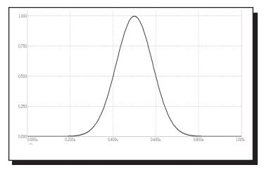
Figure 22-12 GAUSSIAN Waveform for "GAUSSIAN 1 500N 200N 1U"
