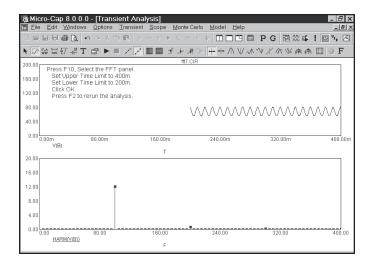
Figure 31-8 The graph without the initial transients
