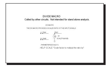
Figure 21-10 DIV macro equivalent circuit
