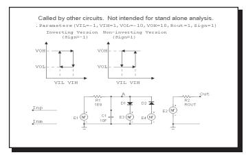
Figure 21-5 COMPARATOR macro equivalent circuit
