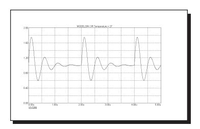
Figure 22-23 Sample waveform for model parameters F=2Meg A=1 DC=1 RP=2U TAU=.4U
