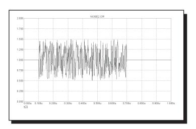
Figure 22-11 NOISE Waveform for "DC 1 AC 1 0 NOISE 2N 1 100N 700N 1"
