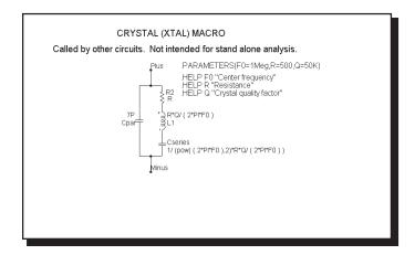
Figure 21-39 XTAL macro equivalent circuit
