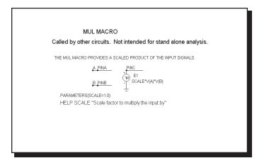
Figure 21-17 MUL macro equivalent circuit
