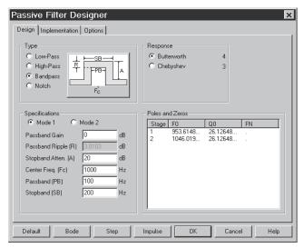
Figure 29-11 The passive filter design panel
