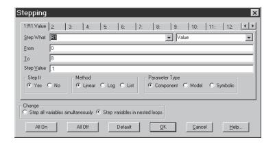
Figure 20-3 R(R1) is stepped from 0 to 8
