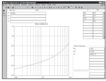
Figure 27-2 The Vbe vs. Ic plot
