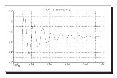
Figure 22-9 Waveform for "SIN 1 1 10Meg 100n 5E6 "  $\,$
