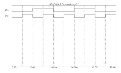
Figure 23-6 Stimulus waveform for example 4
