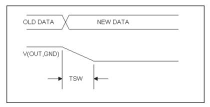
Figure 23-3 DAC timing diagram
