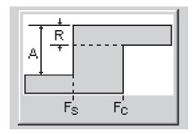
Figure 29-8 High pass filter specifications
