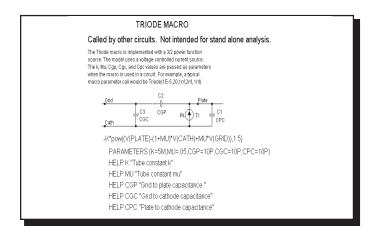
Figure 21-36 TRIODE macro equivalent circuit
