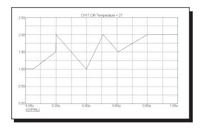
Figure 22-10 Waveform for "PWL 0.05u,1 0.20u,1.5 0.20u,2 0.40u,1 0.51u,2 0.61u,1.5 0.80u,2"
