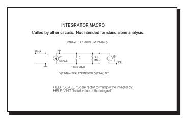
Figure 21-16 INT macro equivalent circuit
