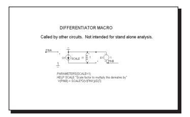
Figure 21-8 DIF macro equivalent circuit
