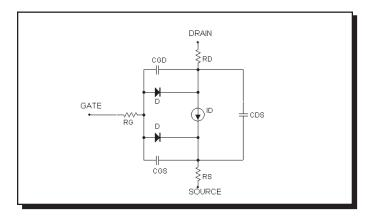
Figure 22-5 The GaAsFET model
