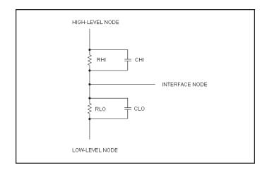
Figure 23-8 N device equivalent circuit
