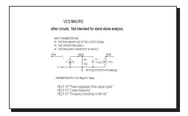
Figure 21-37 VCO macro equivalent circuit
