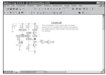
Figure 10-2 Display of initial node voltages
