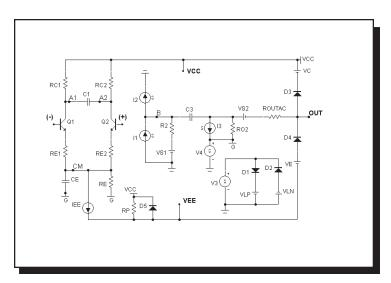
Figure 22-19 The level 3 opamp model with NPN inputs
