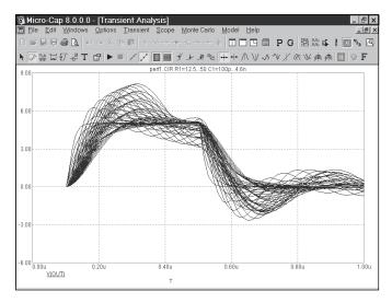
Figure 19-6 Stepping both C1 and R1
