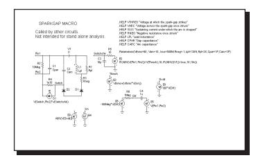
Figure 21-30 SPARKGAP macro equivalent circuit
