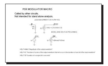
Figure 21-20 PSK macro equivalent circuit
