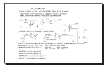
Figure 21-24 RELAY2 macro equivalent circuit
