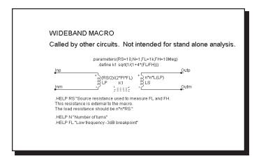
Figure 21-38 WIDEBAND macro equivalent circuit
