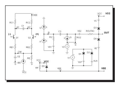
Figure 22-20 The level 3 opamp model with PNP inputs
