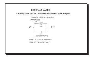
Figure 21-25 RESONANT macro equivalent circuit
