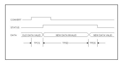
Figure 23-2 ADC timing diagram
