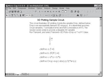
Figure 20-1 The 3D circuit
