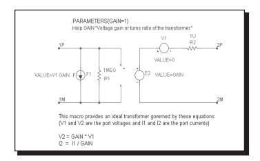
Figure 21-14 Ideal\_Trans2 macro equivalent circuit
