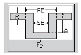
Figure 29-10 Notch filter specifications
