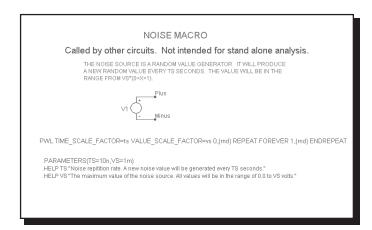
Figure 21-18 NOISE macro equivalent circuit
