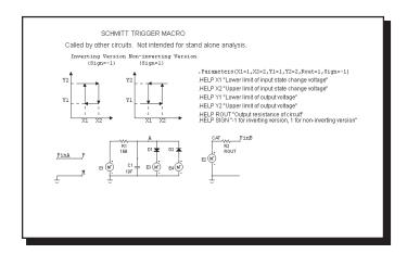
Figure 21-26 SCHMITT macro equivalent circuit
