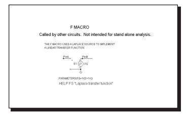
Figure 21-11 F macro equivalent circuit
