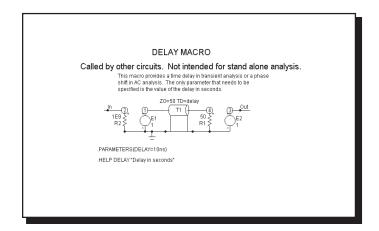
Figure 21-6 DELAY macro equivalent circuit
