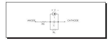
Figure 22-4 Diode model
