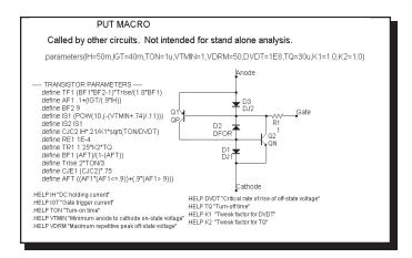
Figure 21-21 PUT macro equivalent circuit
