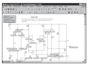
Figure 9-3 1MHz AC voltages in mag, phase (degrees)
