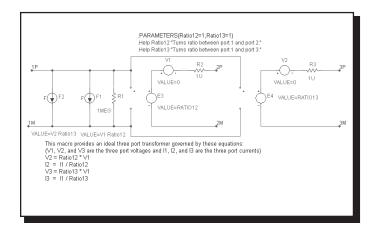
Figure 21-15 Ideal\_Trans3 macro equivalent circuit
