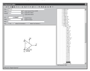
Figure 4-2 The OP09\_AD subcircuit model
