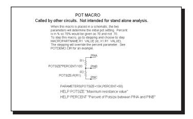
Figure 21-19 POT macro equivalent circuit
