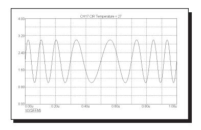
Figure 22-8 Waveform for "SFFM 2 1 8Meg 4 1Meg"
