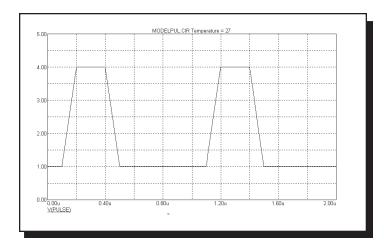
Figure 22-22 Sample waveform for model parameters vzero=1 vone=4 P1=.1u P2=.2u P3=.4u P4=.5u P5=1u
