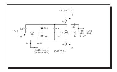
Figure 22-1 Bipolar transistor model
