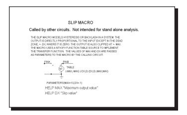
Figure 21-28 SLIP macro equivalent circuit
