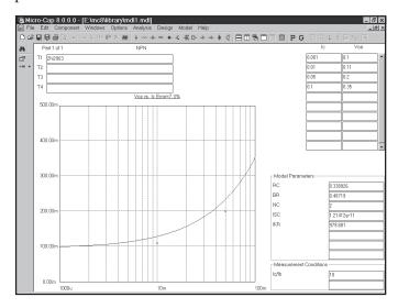
Figure 27-4 The Vce vs. Ic Plot
