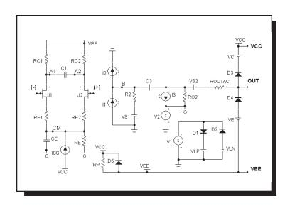
Figure 22-21 The level 3 opamp model with JFET inputs
