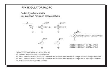
Figure 21-12 FSK macro equivalent circuit
