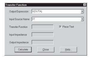
Figure 11-1 The Transfer Function dialog box
