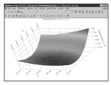
Figure 20-12 The plot of Width vs. L2 and C1
