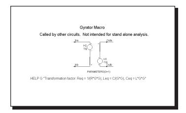
Figure 21-13 GYRATOR macro equivalent circuit
