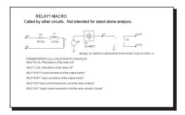
Figure 21-23 RELAY1 macro equivalent circuit
