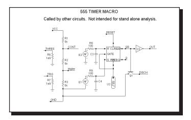
Figure 21-40 555 macro equivalent circuit
