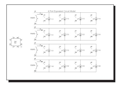
Figure 22-16 Four port equivalent circuit
