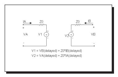
Figure 22-24 Transmission line model
