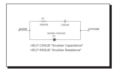
Figure 21-29 SNUBBER macro equivalent circuit
