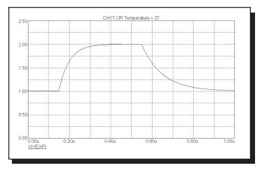
Figure 22-6 Waveform for "EXP 1 2 150n 50n 550n 100n"
