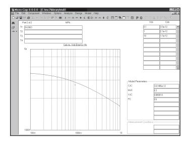
Figure 27-5 The Cob vs. Vcb Plot
