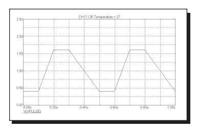
Figure 22-7 Waveform for "PULSE .4 1.6 .1u .1u .2u .1u .5u"
