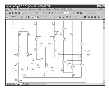
Figure 13-2 Distortion sample circuit
