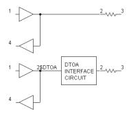
When an analog node is connected to a digital node with both input and output pins connected to it, a new digital node, 2\$DTOA, is created and assigned to the digital node. An interface circuit is inserted between the new digital node and the analog node.
