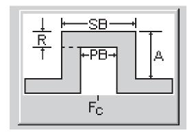
Figure 29-9 Bandpass filter specifications
