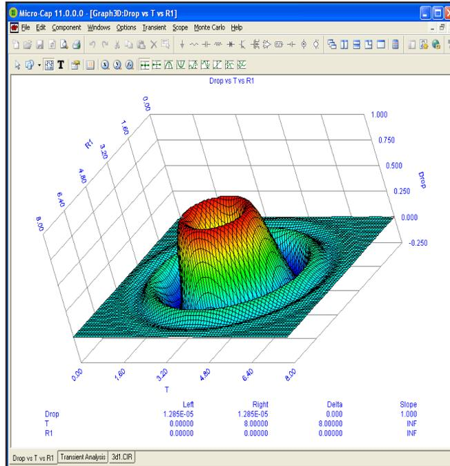
**Figure 23-10 The 3D plot in Cursor mode**
