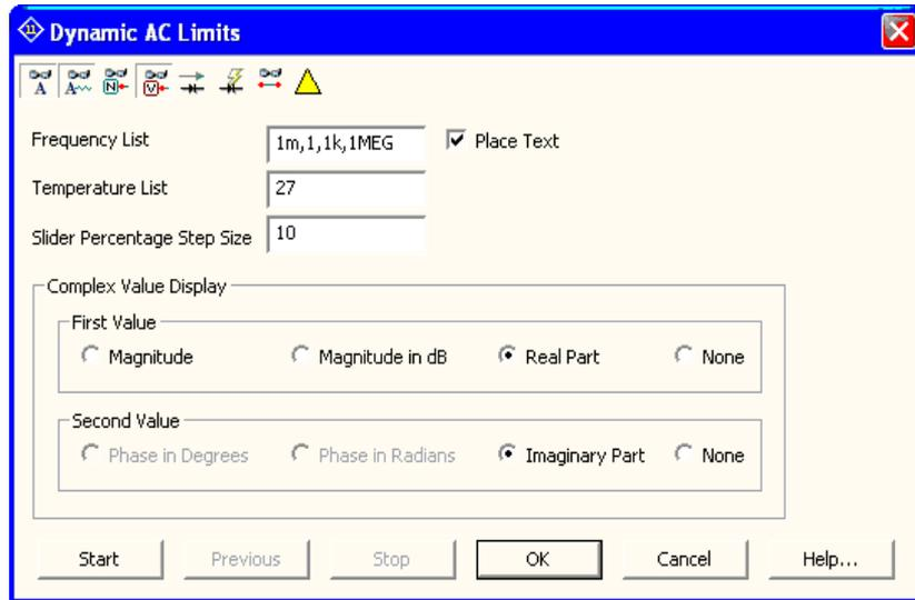
**Figure 9-1 The Dynamic AC Analysis Limits display**
