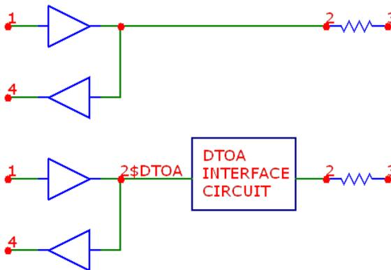
When an analog node is connected to a digital node with both input and output pins connected to it, a new digital node, 2\$DTOA, is created and assigned to the digital node. An interface circuit is inserted between the new digital node and the analog node.
