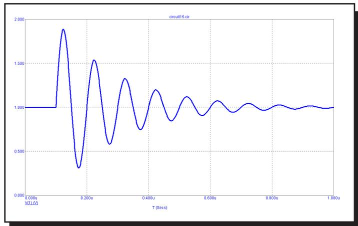
Figure 25-13 Waveform for "SIN 1 1 10Meg 100n 5E6"
