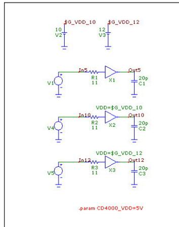
**Figure 26-10 CD4000 Devices Using Different Power Supplies**
