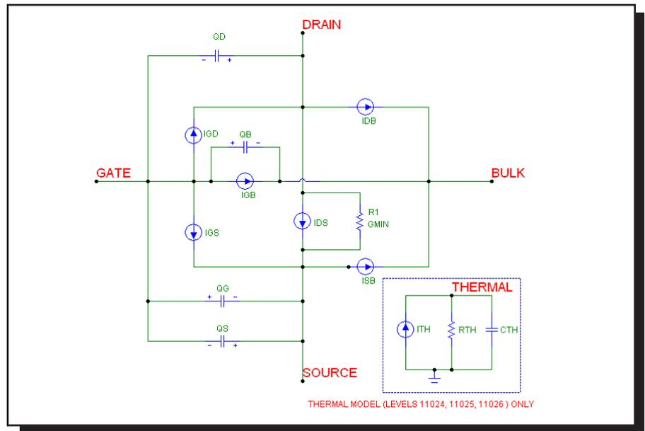
**Figure 25-21 Electrical model of Philips Model 11**
