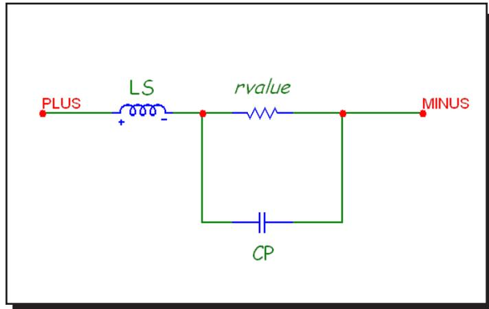
Figure 25-33 Resistor model
