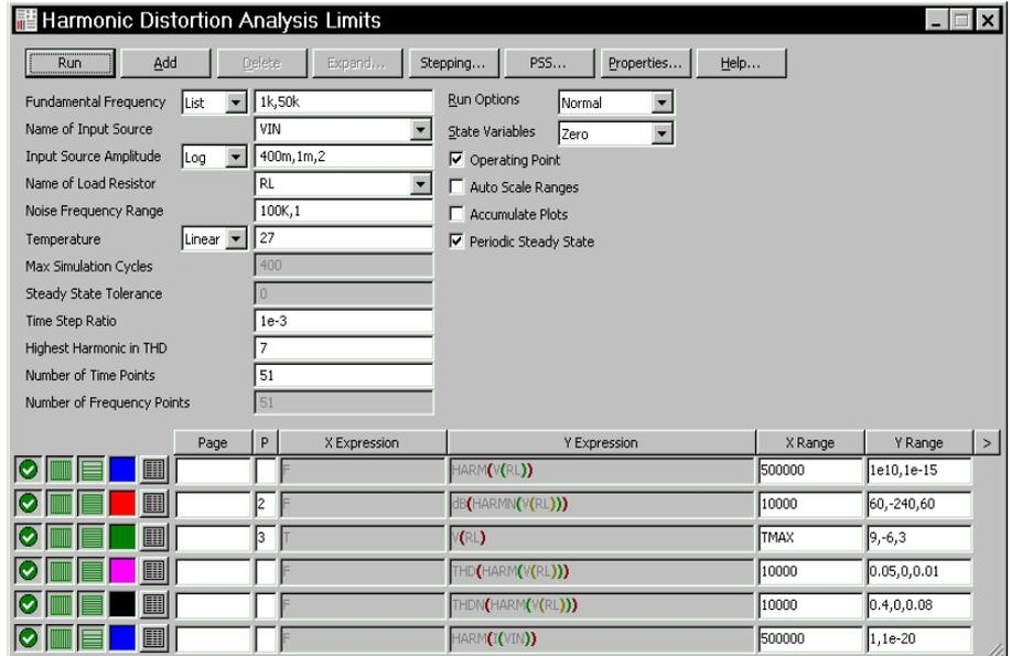
**Figure 13-1 Harmonic Distortion Analysis Limits dialog box**
