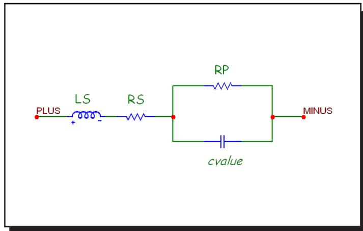
Figure 25-4 Capacitor model
