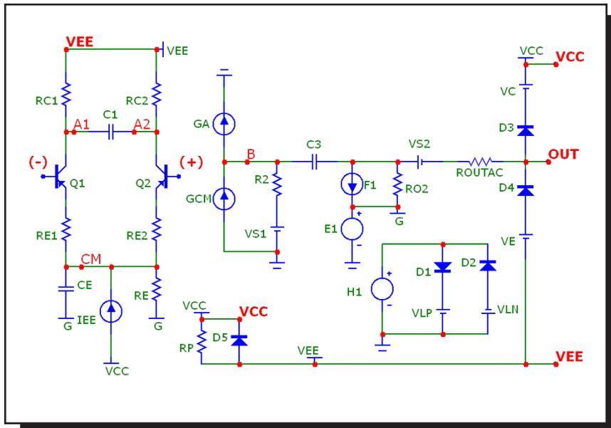
Figure 25-30 The level 3 opamp model with PNP inputs
