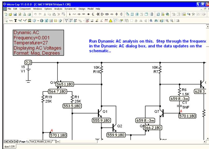
Figure 9-3 AC voltages in mag, phase (degrees)
