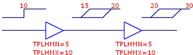
Ambiguity can do more than just fuzz up the signal edges. It can catastrophically alter simulation results. In the circuit below, the ambiguous D input signal makes the output 'X' since there are two possible outcomes. If the clock completes its rise before the D input changes, the Q output remains '0'. If the clock completes its rise after the D input changes, the new '1' state is loaded and the Q output becomes '1'.
