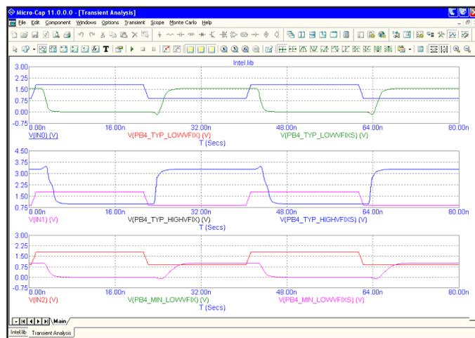
**Figure 31-3 Sample Golden Waveforms plots**
