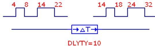
This type of delay is useful when you want to shift a signal by some fixed delay value without removing any of its narrow pulses. Only the DLYLINE device uses transport delay. All delay parameters of all other devices are treated as inertial, except when inertial cancellation is disabled.
