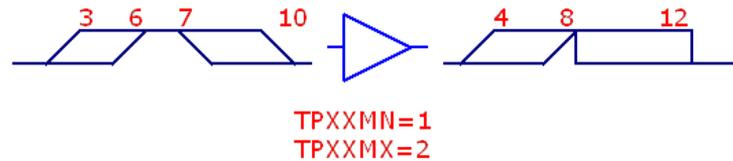
At 7, the simulator attempts to schedule the 'F' state at 8 (7+1). But the '1' state is already scheduled to occur on the output at 8 (6+2). Since this is ambiguous, the simulator signals a hazard with an 'X' at 8.
