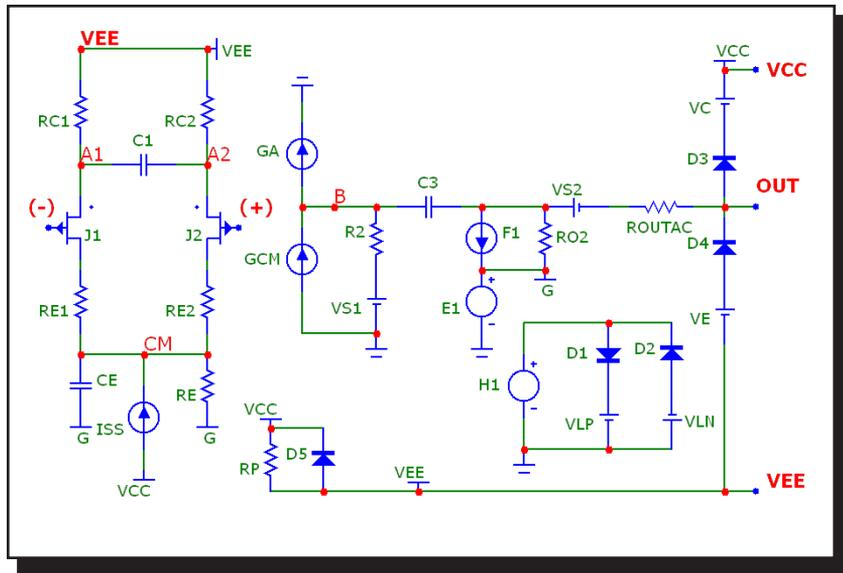
Figure 25-31 The level 3 opamp model with JFET inputs
