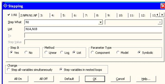
**Figure 9-10 The Stepping dialog box for text stepping the N1 variable**
