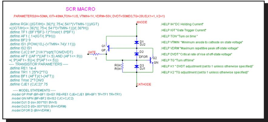
**Figure 24-44 SCR macro circuit**
