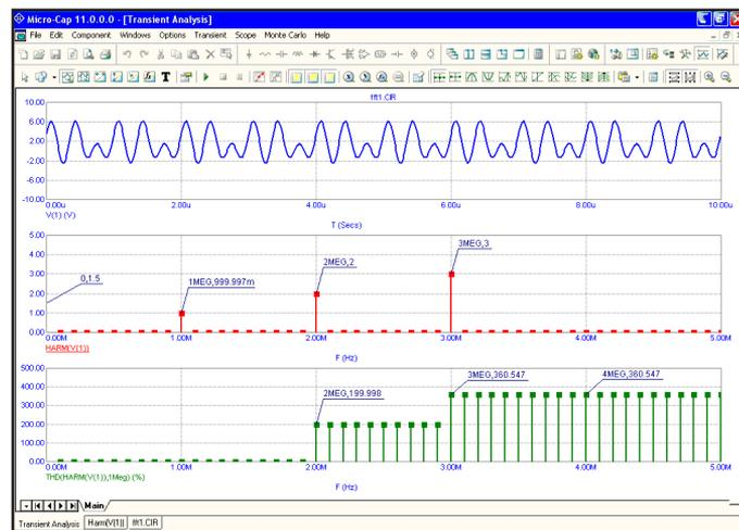
Figure 34-5 The graph with tmax = 10u and FR = 1MHz
