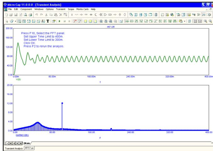
**Figure 34-7 The graph with the initial transients**
