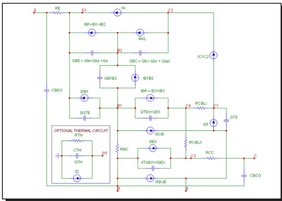
**Figure 25-2 Mextram bipolar transistor model**
