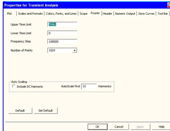
**Figure 34-6 The Fourier control panel**
