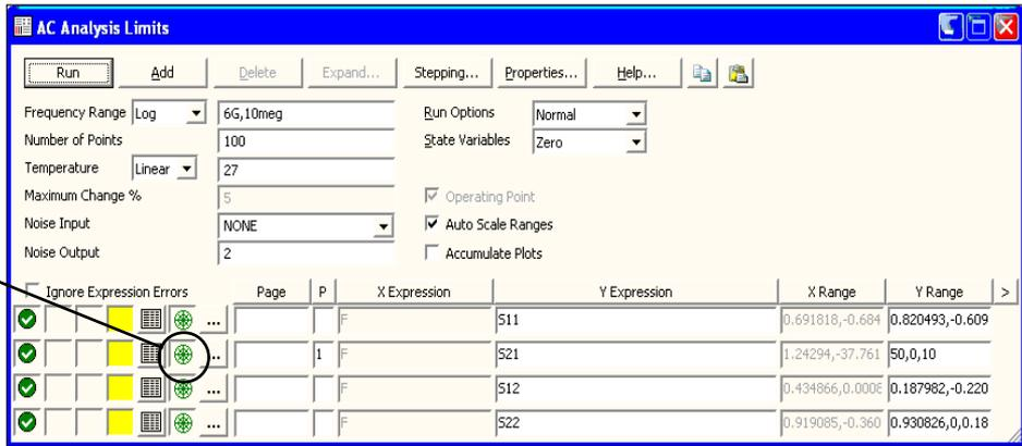
Figure 5-14 Analysis limits for a polar plot
