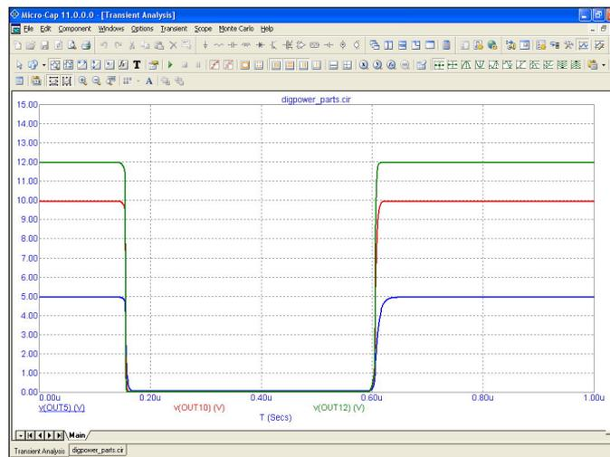
**Figure 26-11 Transient Output Using Different Power Supplies**
