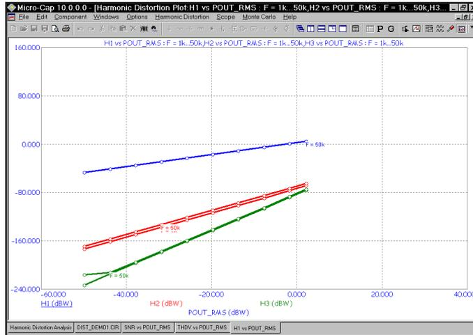
Figure 13-4 Harmonic Power vs. PIN
