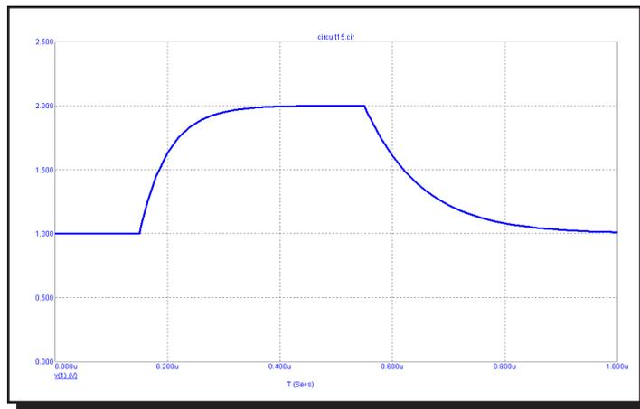
Figure 25-10 Waveform for "EXP 1 2 150n 50n 550n 100n"
