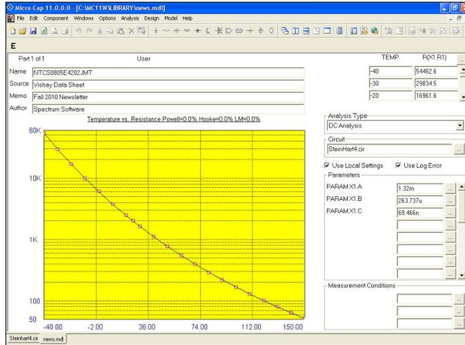
**Figure 30-13 Final Optimization Results for the 2K Thermistor**
