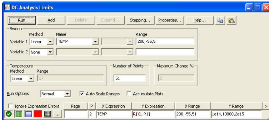
**Figure 30-10 DC Analysis Limits for the Steinhart Circuit**
