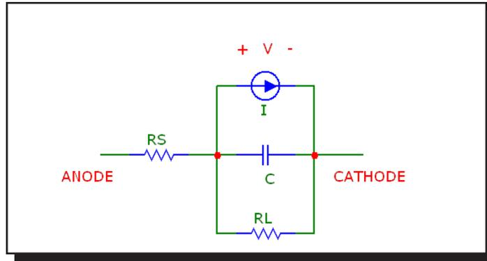
Figure 25-7 Diode model
