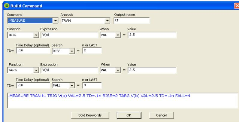
**Figure 2-23 .Measure command with TRIG and TARG**
