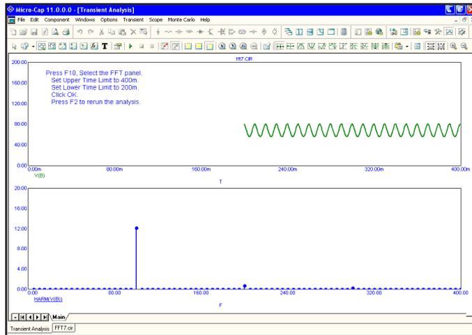
**Figure 34-8 The graph without the initial transients**
