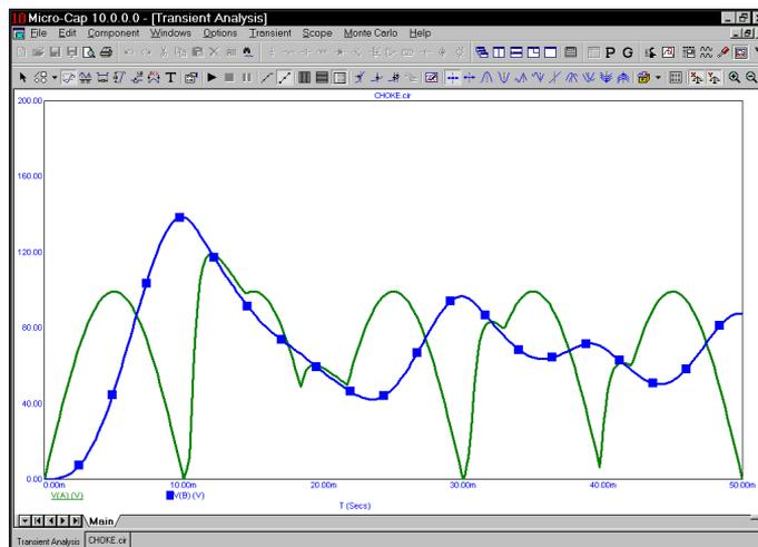
**Figure 7-2 Transient analysis of the CHOKE circuit**
