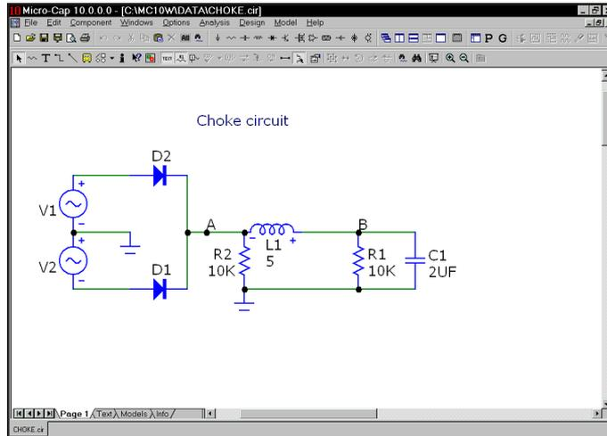
**Figure 7-1 The CHOKE circuit**
