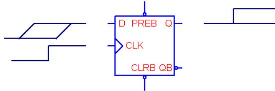
Since there are two possible opposite states for Q depending upon when the D input changes, the Q output is assigned 'X' to reflect the uncertainty.
