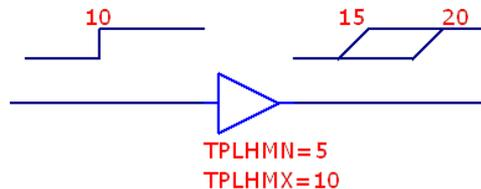
If MNTYMXDLY is 4, the resulting worst-case run produces a rising state at 15 since the minimum low to high delay is 5. The "TPLHMN=5" says that the delay is at least 5. It may be more. The "TPLHMX=10" says that the delay is at most 10. It may be less. The rising state between 15 and 20 reflects the uncertainty.
