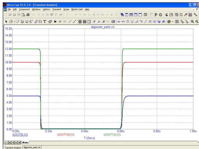
**Figure 23-11 Transient Output Using Different Power Supplies**
