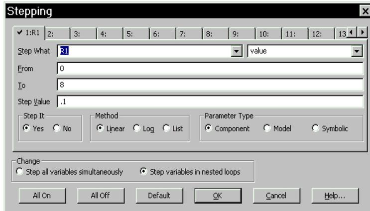
**Figure 20-3 R(R1) is stepped from 0 to 8**
