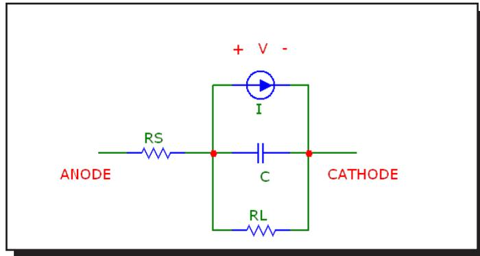
Figure 22-7 Diode model
