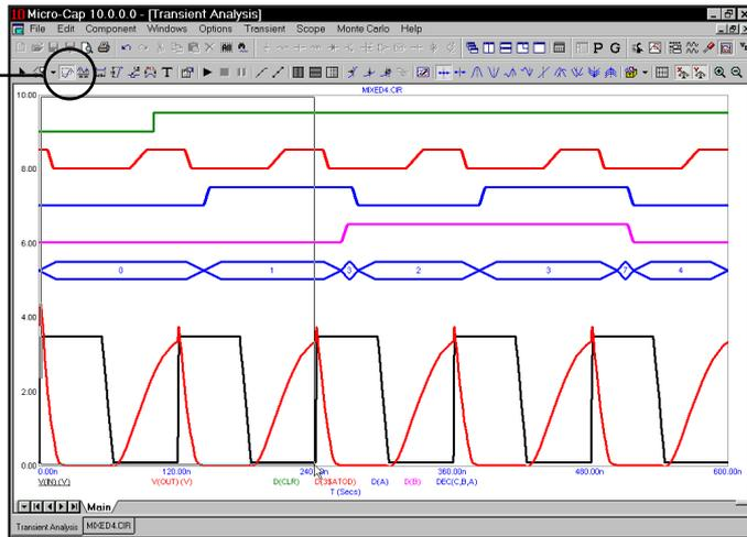
Figure 2-4 Using the mouse to magnify a waveform
