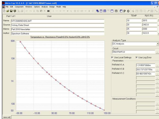
**Figure 27-13 Final Optimization Results for the 2kOhm Thermistor**
