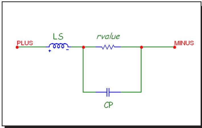
Figure 22-33 Resistor model
