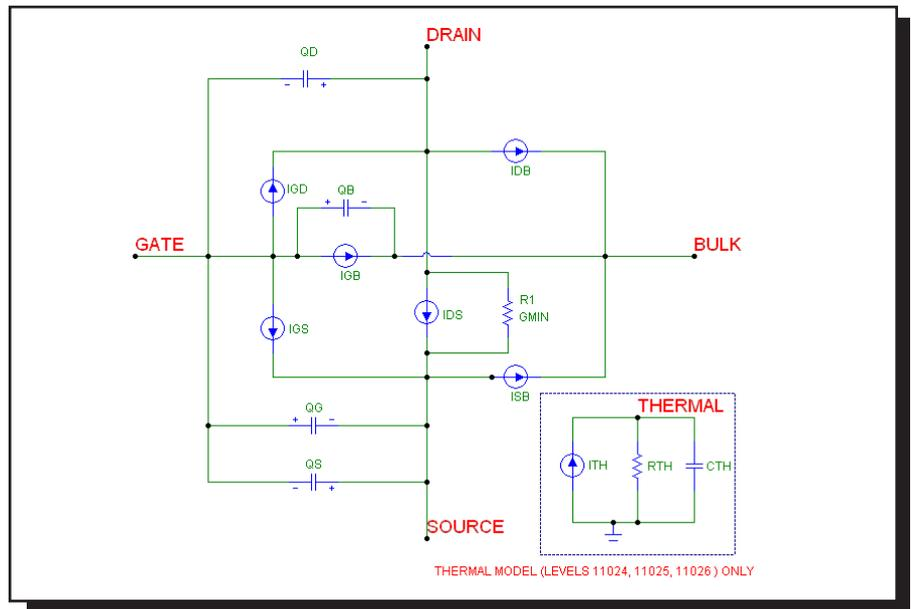
Figure 22-21 Electrical model of Philips Model 11
