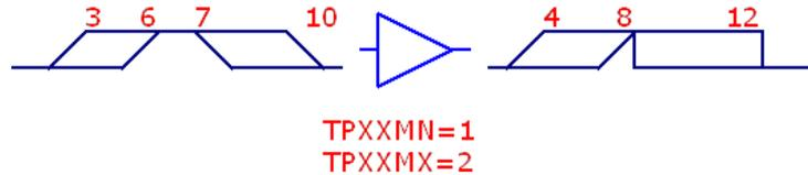
At 7, the simulator attempts to schedule the 'F' state at 8 (7+1). But the '1' state is already scheduled to occur on the output at 8 (6+2). Since this is ambiguous, the simulator signals a hazard with an 'X' at 8.
