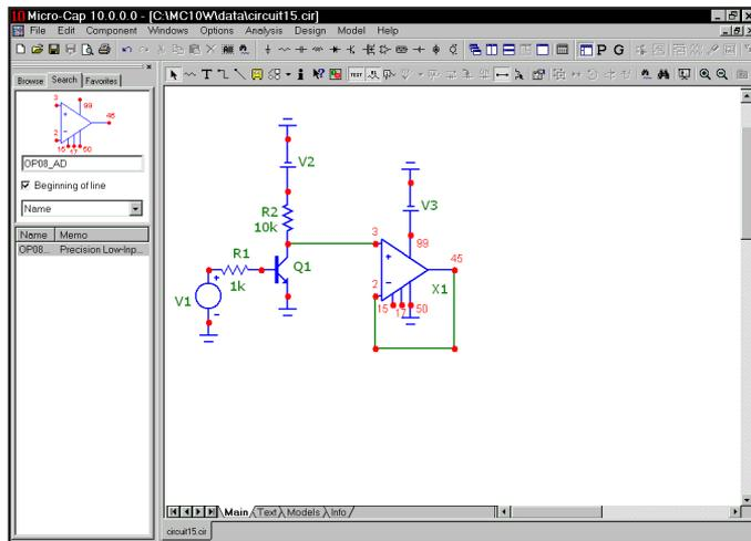
**Figure 3-8 The circuit after wiring the OP08**
