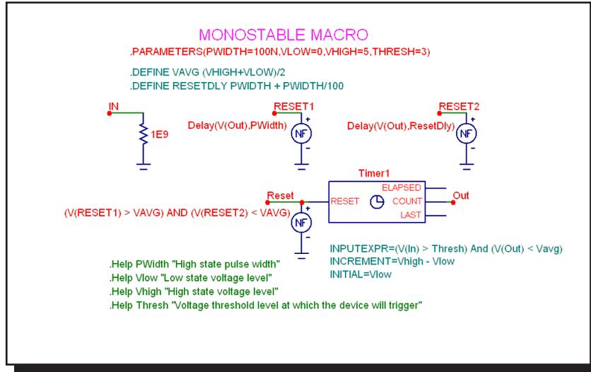
**Figure 21-27 MONOSTABLE macro circuit**
