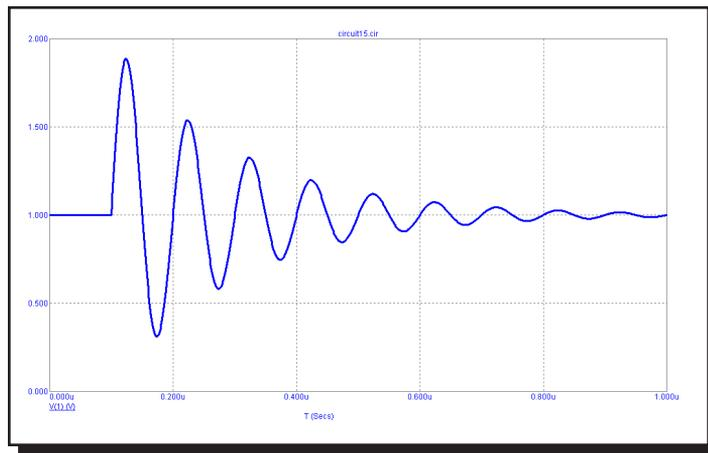
**Figure 22-13 Waveform for "SIN 1 1 10Meg 100n 5E6"**
