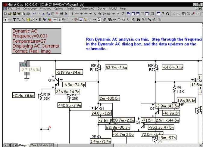
Figure 9-6 AC currents at V1 = 13.5V DC
