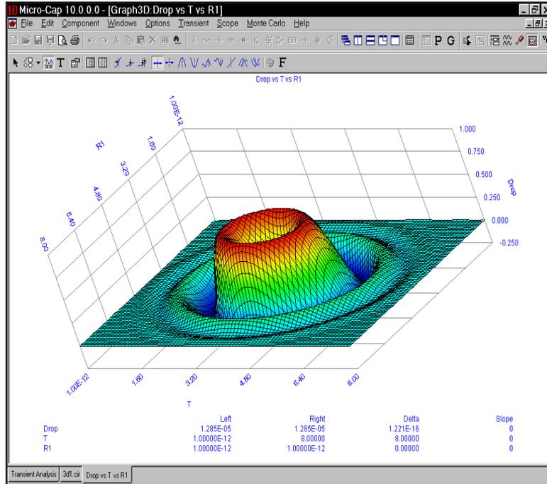
**Figure 20-10 The 3D plot in Cursor mode**
