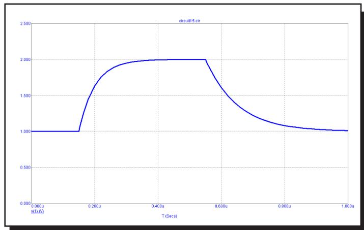
Figure 22-10 Waveform for "EXP 1 2 150n 50n 550n 100n"
