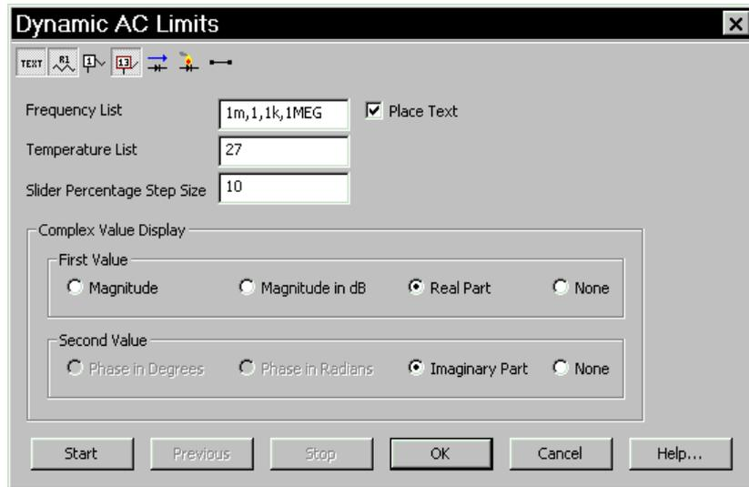
**Figure 9-1** The Dynamic AC Analysis Limits display
