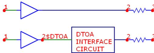
When the digital node is an output node, a new digital node, 2\$DTOA, is created and assigned to the digital output, and the DTOA interface circuit, specified by the I/O model statement IO\_LEVEL parameter, is inserted between the new digital output node and the analog node.
