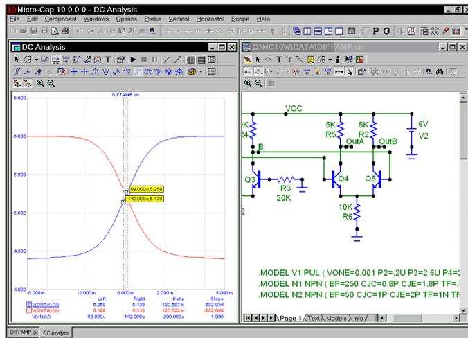
Figure 8-10 Using the cursors to find the peak gain
