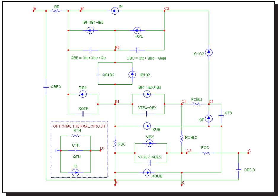
Figure 22-2 Mextram bipolar transistor model
