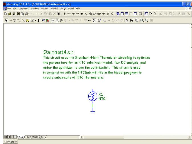
**Figure 27-9 NTC Thermistor Optimization Test Circuit**
