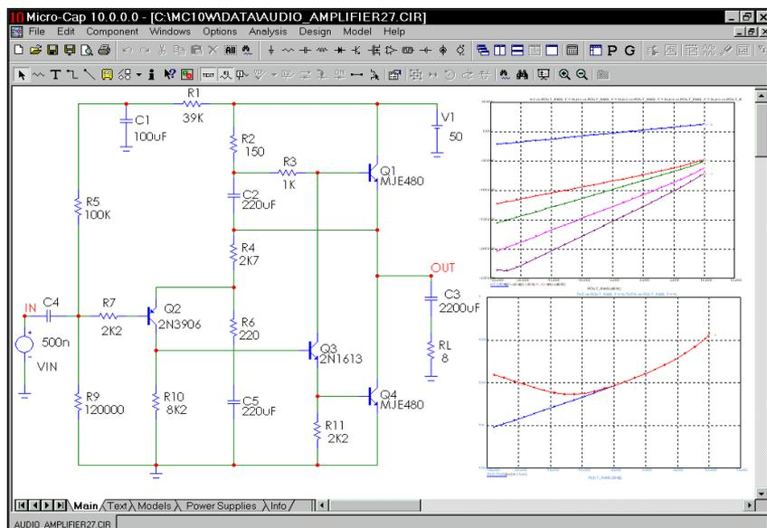
**Figure 2-7** A circuit with two WMF picture files
