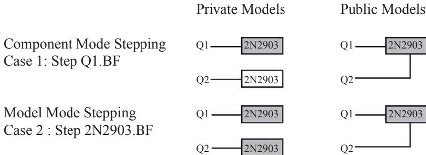
The shaded models are changed by stepping. In case 1, we are stepping Q1.BF. In this case we step the model that Q1 points to. When the libraries are private, then the model pointed to by Q1 would be stepped and that pointed to by Q2 would not be stepped. They point to distinct model locations, even though they use the same model name. When the libraries are public, stepping the model pointed to by Q1 also steps the model pointed to by Q2 since they point to the same model location.
