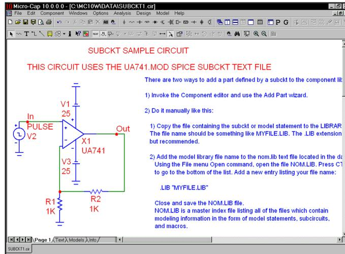
Figure 12-4 Using the subckt component
