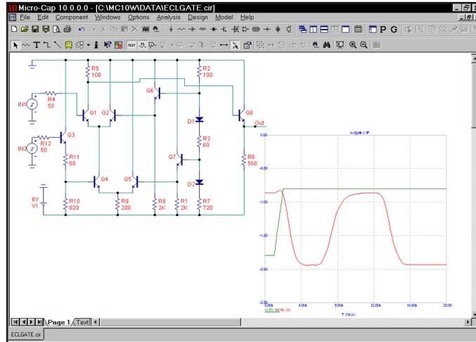
**Figure 13-7 Adding a WMF of the analysis plot**
