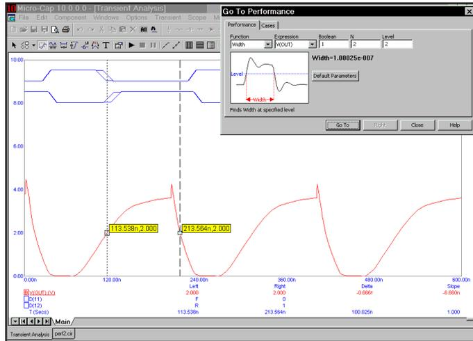
**Figure 7-21 Measuring the pulse width**
