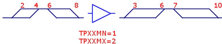
As the signal passes through additional stages, the uncertainties can accumulate to the point where parts of the signal are ambiguous, as in this example:
