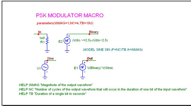
**Figure 21-35 PSK macro circuit**
