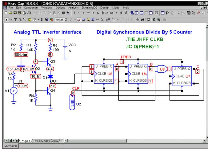
**Figure 2-6 Operating point node voltages and states**
