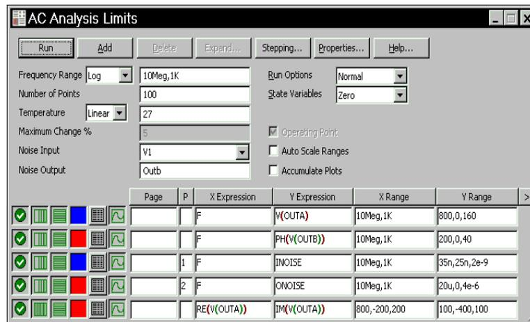
Figure 5-8 The Analysis Limits for Noise plots
