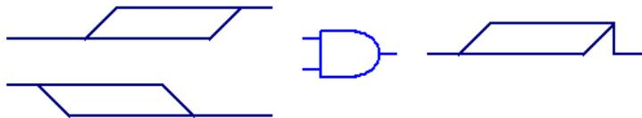
hazard. It should be interpreted as a possible short pulse, extending no longer than the overlap of the uncertainty portions of the two input signals.
