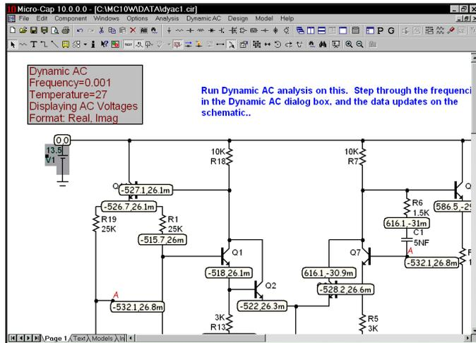
Figure 9-5 AC voltages at V1 = 13.5V DC
