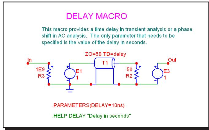
**Figure 21-12 DELAY macro circuit**
