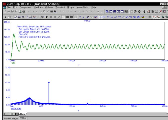
**Figure 31-7 The graph with the initial transients**
