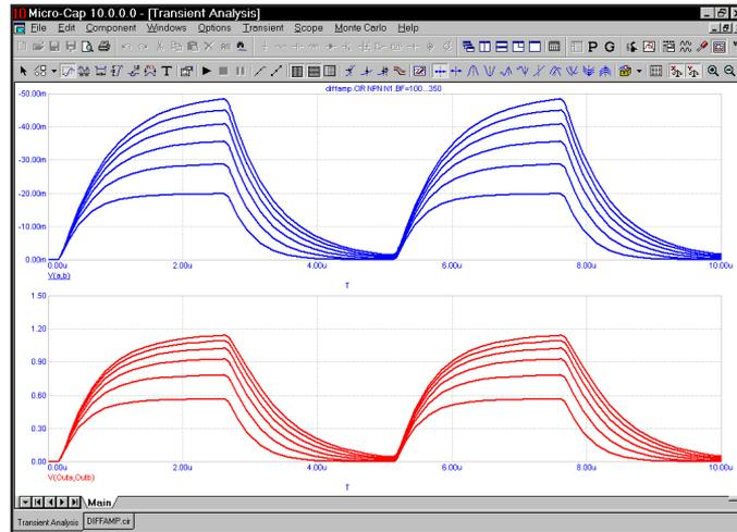
**Figure 9-2 Stepping BF in four transistors simultaneously**
