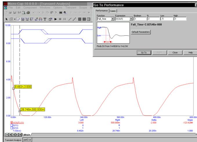
Figure 7-19 Measuring fall time
