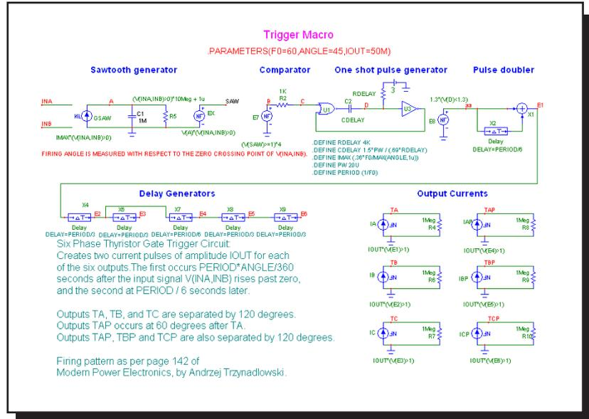
Figure 21-52 TRIGGER6 macro circuit
