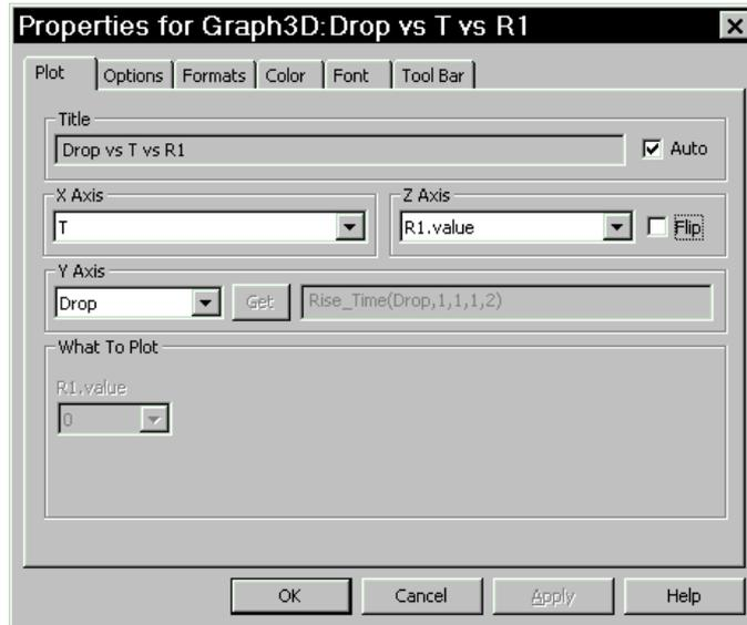
**Figure 20-6** The Plot panel of the 3D dialog box
