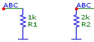
Naming is done by dropping a piece of text on a node or by double-clicking on a wire and changing its node name. Both procedures name the node.
