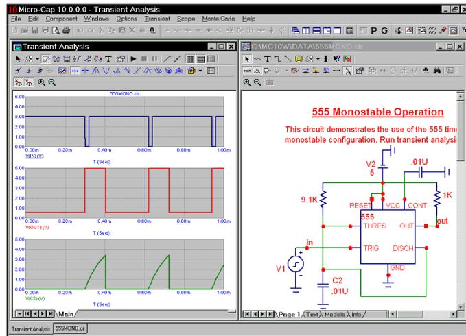
Figure 4-15 Transient analysis of 555MONO
