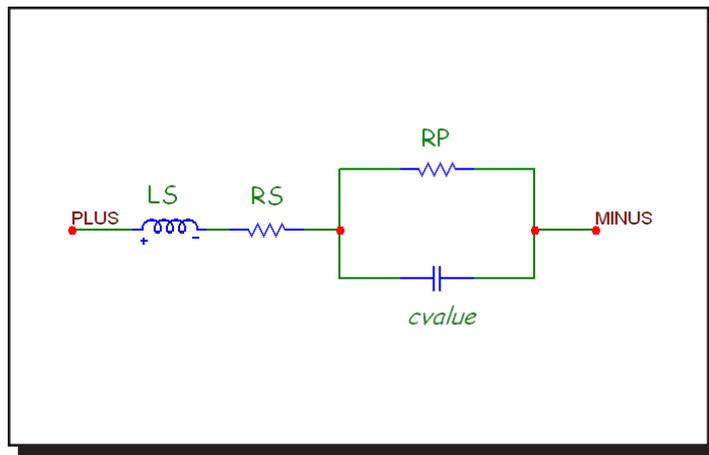
Figure 22-4 Capacitor model
