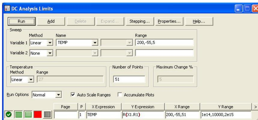
**Figure 27-10 DC Analysis Limits for the Steinhart Circuit**
