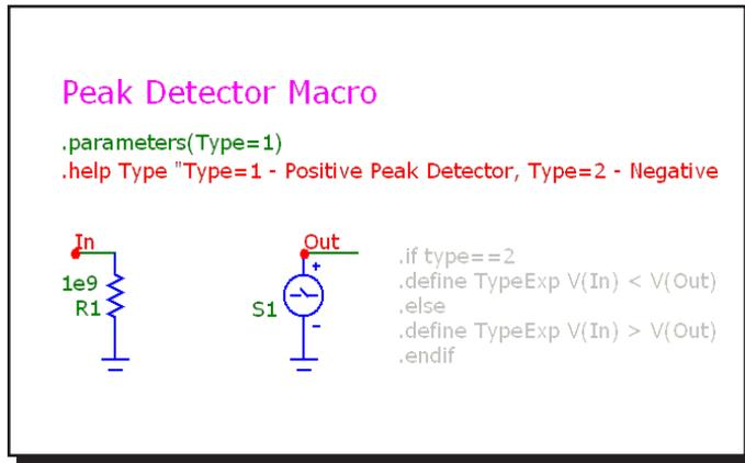
**Figure 21-30 Peak Detector macro circuit**
