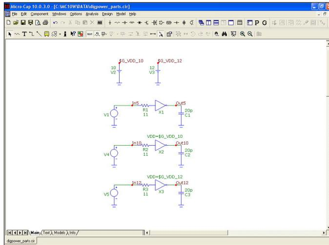
**Figure 23-10 CD4000 Devices Using Different Power Supplies**
