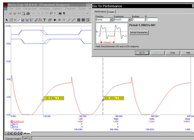
Figure 7-20 Measuring the pulse period
