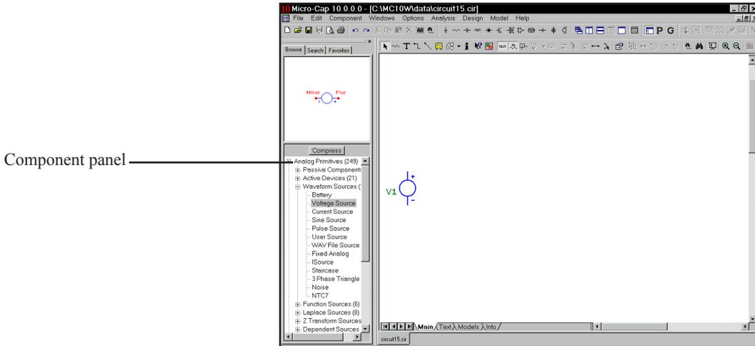
**Figure 3-1** Selecting a part from the Component panel
