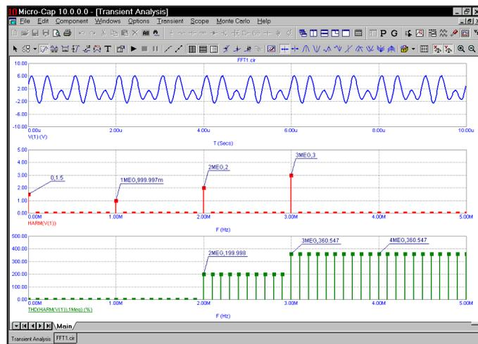
**Figure 31-5** The graph with tmax = 10u and FR = 1MHz
