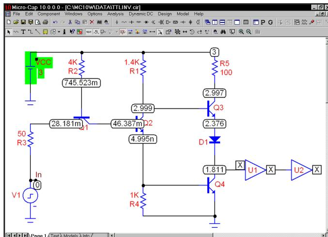
Figure 10-3 Display of voltages at the switching point
