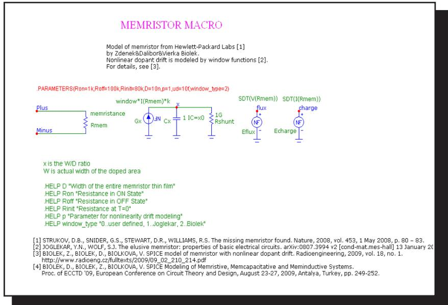
**Figure 21-25 Memristor macro circuit**
