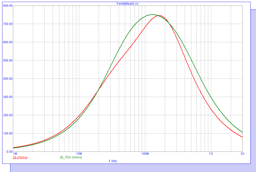
Fig. 17 - Micro-Cap model versus TDK model
