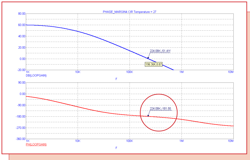
Fig. 7 Phase margin with CC = 80pF = 180 - 181.55 = -1.55 degrees = unstable
