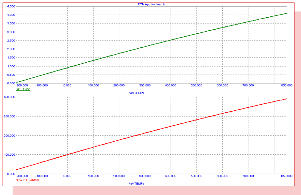
Fig. 8 - RTD interface circuit DC analysis
