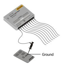
Figure 2-11 Connect to the ground
