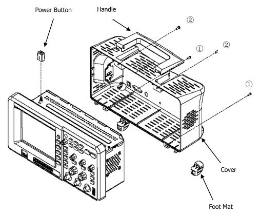
Figure 5-2 Disassemble and assemble the cover
