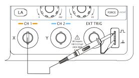
Figure 2-6 Connect the probe compensator
