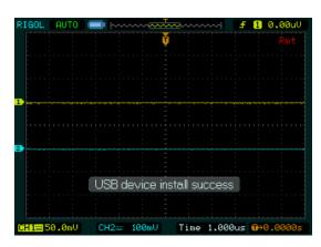
Figure 3-2 Successful prompt of USB interface connection
