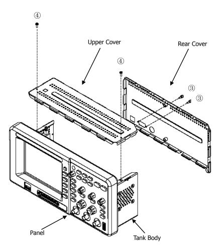
Figure 5-3 Disassemble and assemble the upper and rear covers
