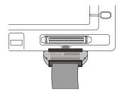
Figure 2-8 Connect the digital probes to oscilloscope
