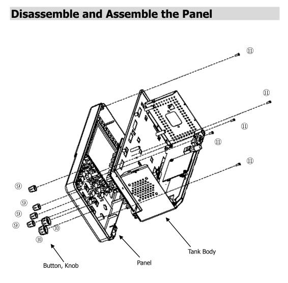
Figure 5-5 Disassemble and assemble the panel
