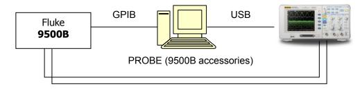
Figure 3-14 Connect the testing device
