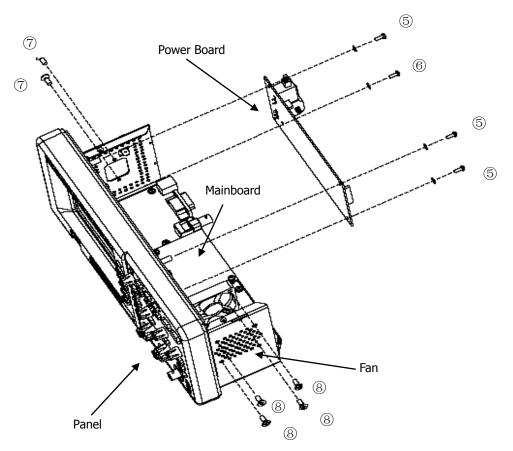
Figure 5-4 Disassemble and assemble the power board and the fan
