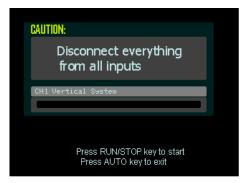
Figure 4-1 Self-Calibration interface
