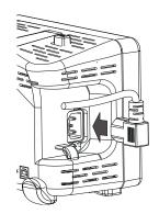
Figure 2-1 Connect the power cord
