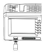
Figure 3-1 Connect the U disk
