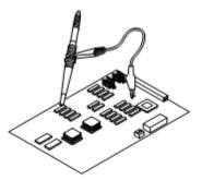
Figure 2-4 Connect probe to circuit
