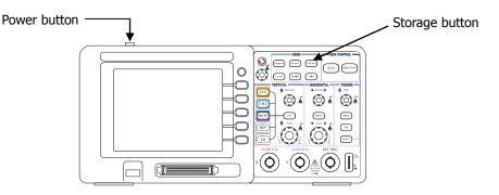
Figure 2-2 Power-on inspection
