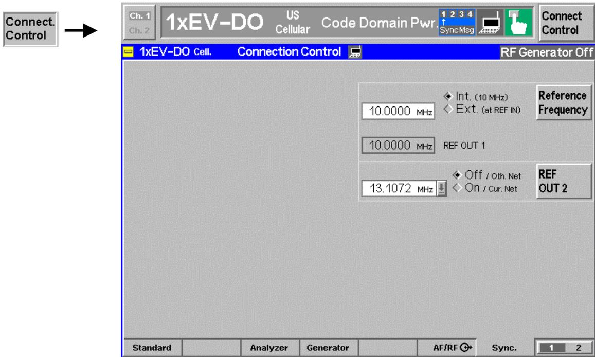
Figure 4-31 Connection Control – Synchronization
