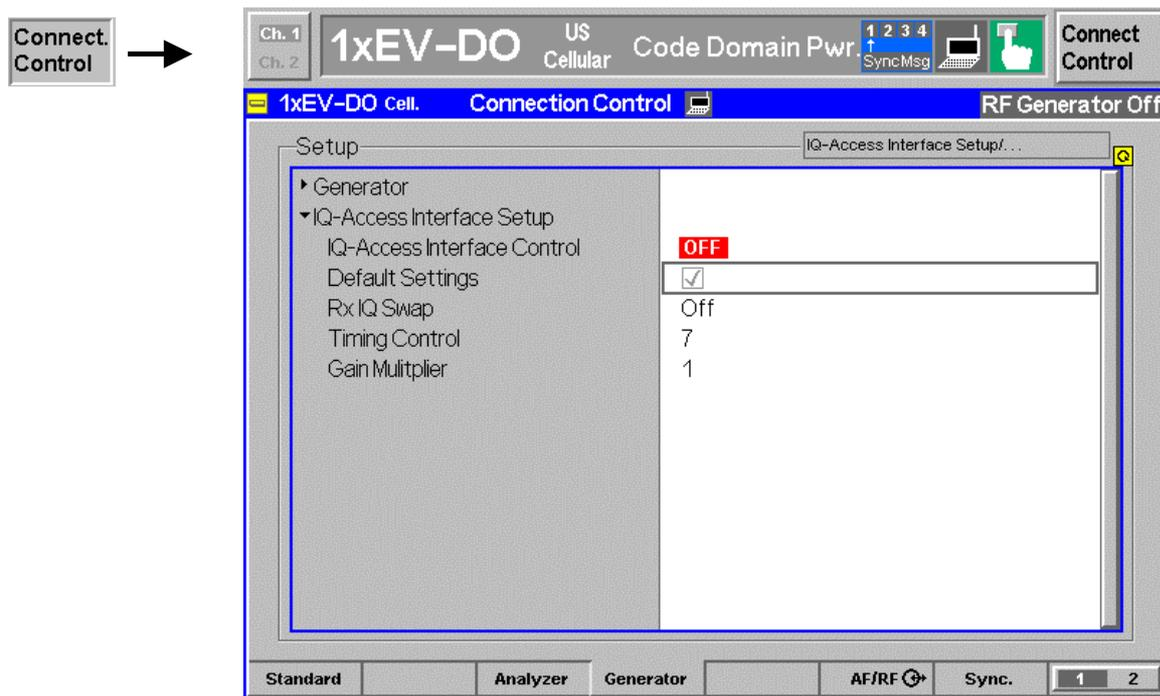
Figure 4-29 Connection Control – IQ-Access Interface Setup
