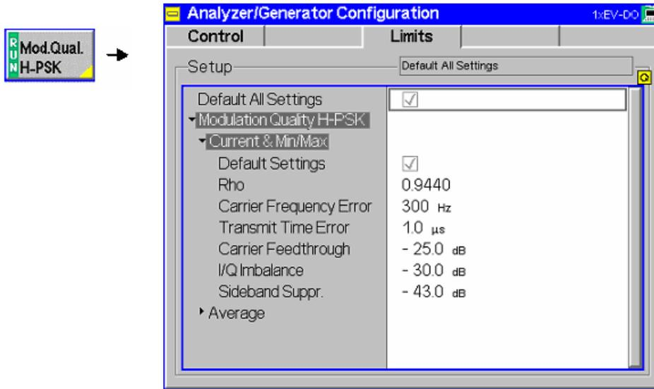
Figure 4-5 Modulation Configuration – Limits
