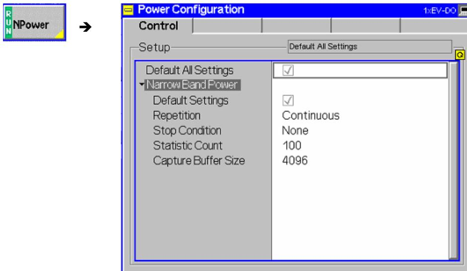
Figure 4-8 Power Configuration – Control
