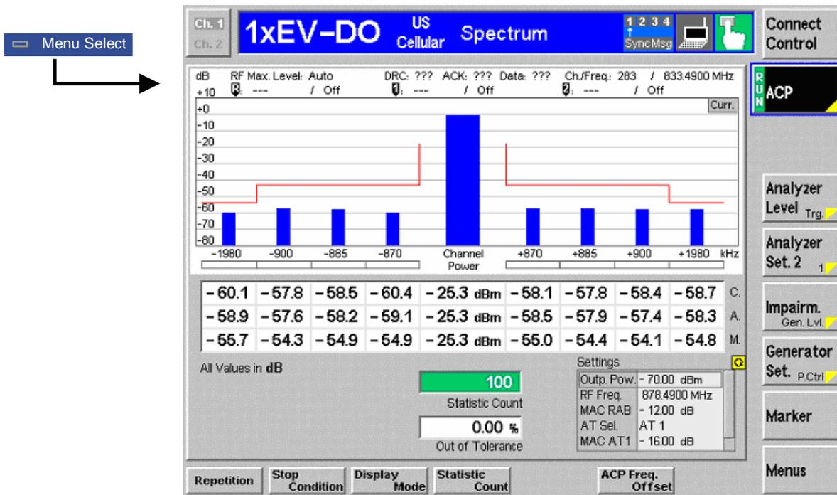
Figure 4-16 Measurement menu Spectrum
