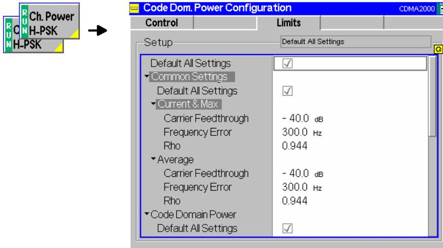
Figure 4-25 Code Domain Power Configuration – Limits
