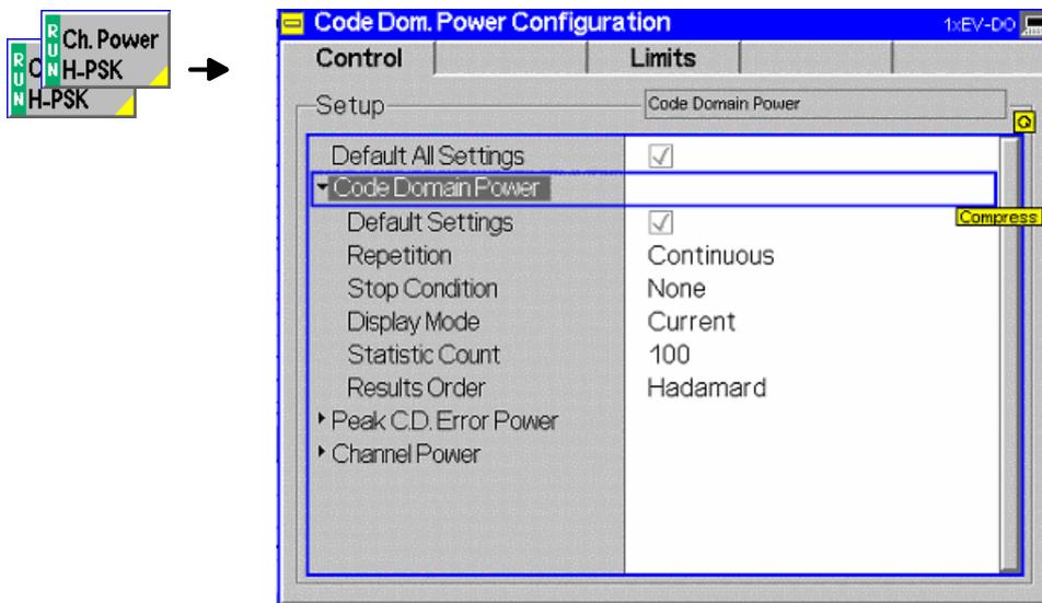
Figure 4-24 Code Domain Power Configuration – Control
