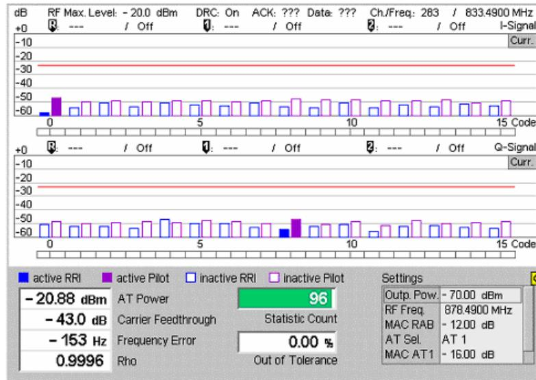
Figure 4-22 Display of measurement results (Code Domain Error Power screen)
