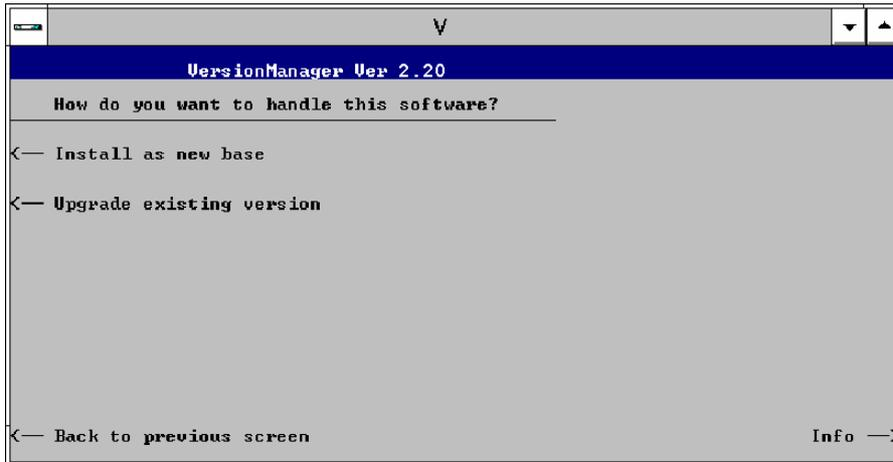
*Note:* This dialog is skipped if the new base software version is not compatible with any of the existing configurations. An incompatible new base software must be installed as a new base software.
