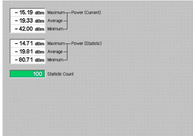
Figure 4-7 Display of results (NPower)
