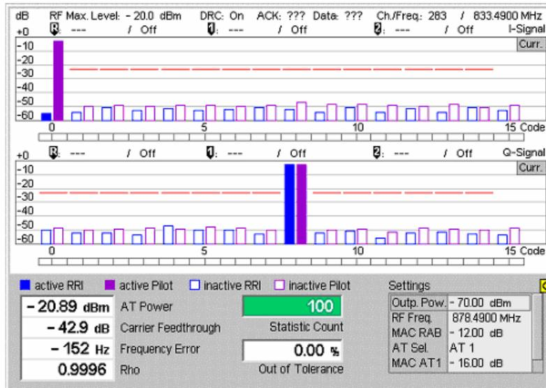
Figure 4-21 Display of measurement results (Code Domain Power screen)
