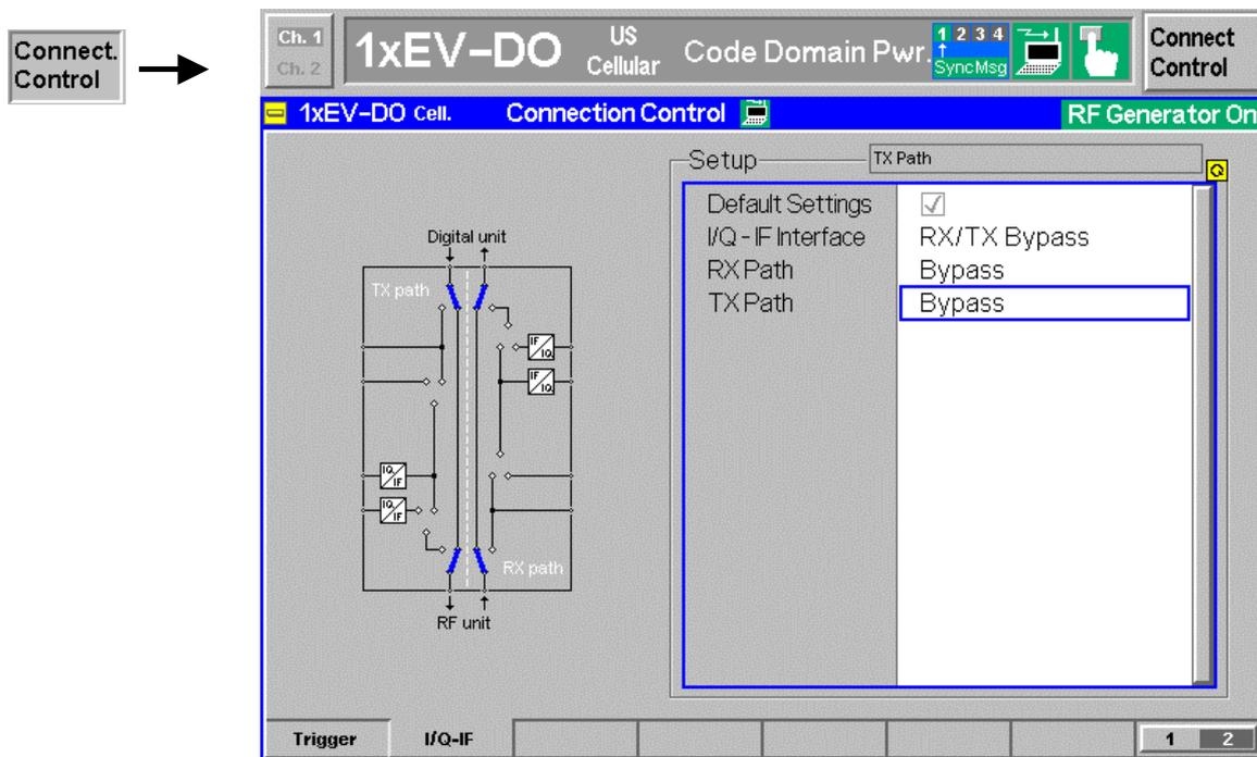
Figure 4-33 Connection Control – I/Q-IF
