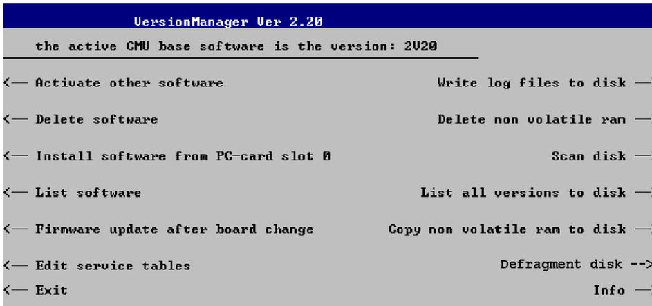
Softkey no. 5 on the left softkey bar, *Install software...*, is used to install new software from an external storage medium. The CMU automatically recognizes the storage medium and indicates the corresponding slot number: Slot 0 or 1 denotes the left or right slot of the PCMCIA interface. If a floppy disk is used, the menu option reads *Install software version <version> from floppy*.
