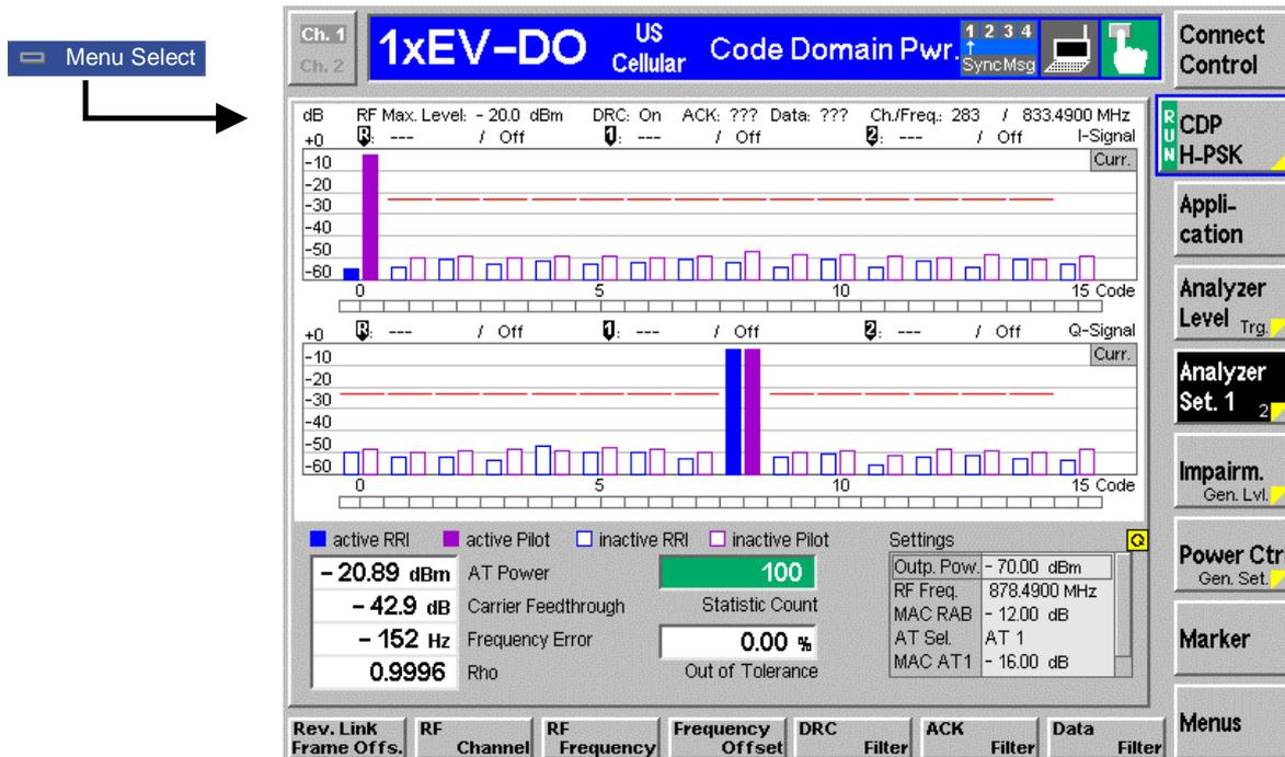
Figure 4-20 Code Domain Power measurement menu
