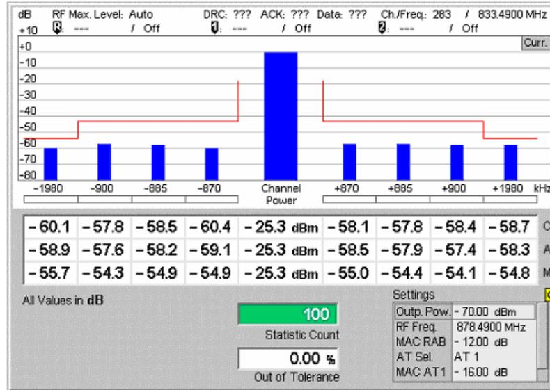
Figure 4-17 Display of results (Analyzer/Generator)
