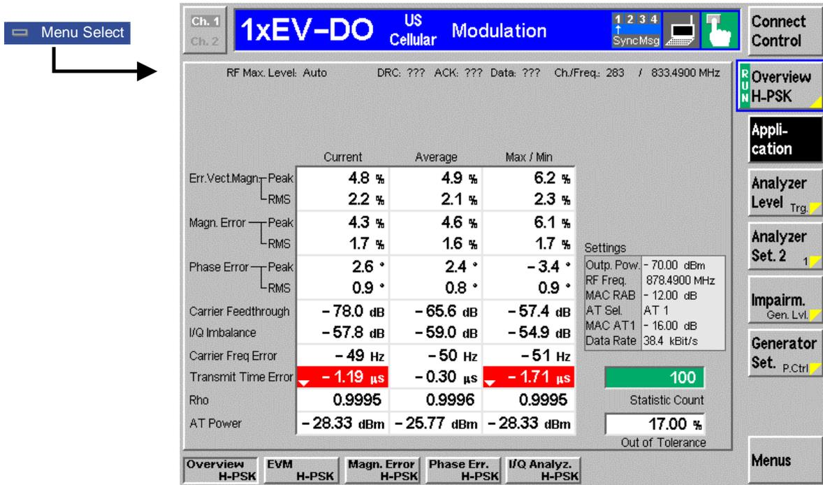
Figure 4-10 Measurement menu Modulation
