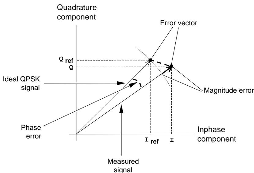
Figure 4-9 Modulation errors
