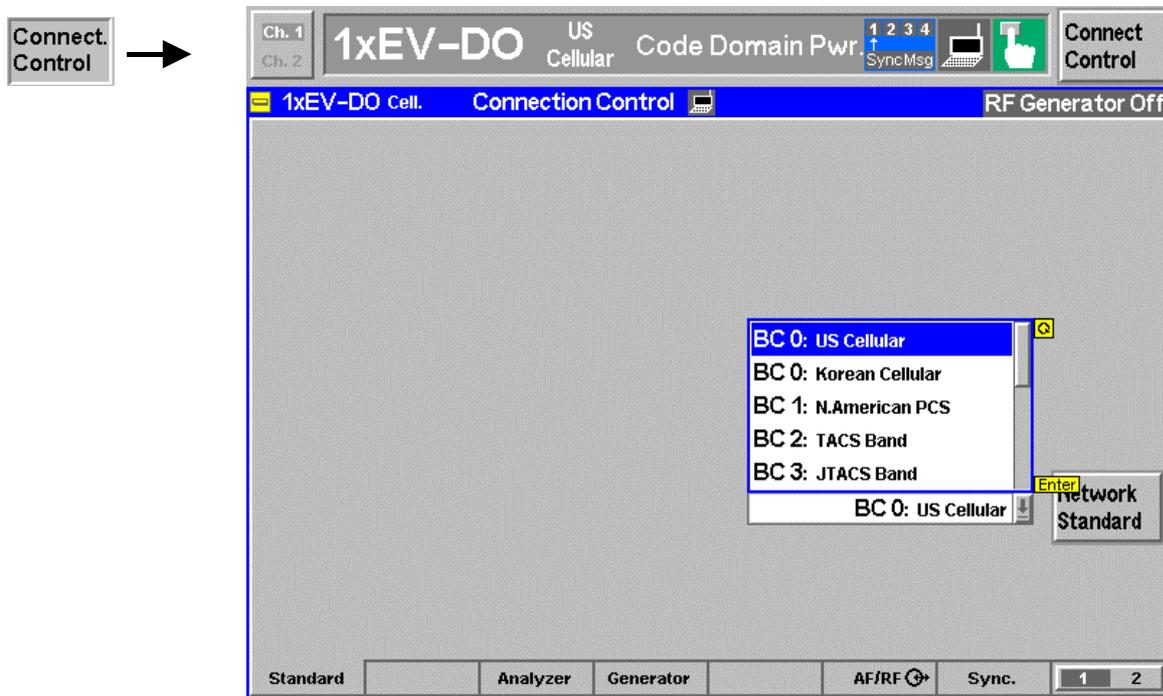
Figure 4-26 Connection Control – Standard
