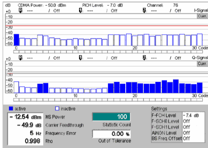
Figure 4-52 Display of measurement results (Code Domain Error Power screen)
