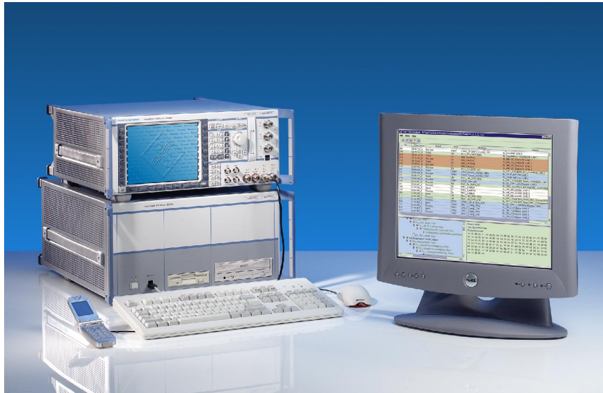
Fig. 17: Protocol Tester R&S CRTU-W for WCDMA/HSDPA
