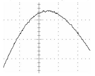
The value to RMS \* $\sqrt{2}$  yields much more stable values for the level search since it "filters out" any interference. These values are then, however, lower than the displayed peak value. Consequently, the audio level found using the level search is higher than that for instruments which only provide peak weighting.
