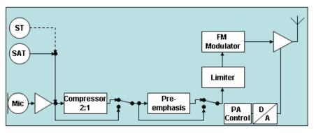
In the AMPS phone, the amplified audio signal from the microphone first enters a "compressor". The reference deviation for AMPS is 2.9 kHz. This means that the audio signal should generate a deviation of 2.9 kHz at fullscale level. The relationship between audio signal level and deviation is, however, not linear. A 6-dB-lower input level attenuates the deviation by only 3 dB. A 6-dB-higher audio signal amplifies the deviation by only 3 dB.
