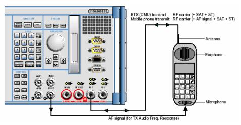
RF2 is normally used for the bidirectional RF connection. It is also possible to use the RF1 connector; however, the dynamic range of this input (and output) is less suitable for testing AMPS phones. There is one exception: if
