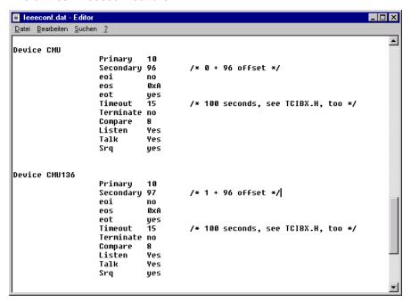
The test software initialises the devices "CMU" and "CMU136" by sending the CMU-specific initialisation strings from the CRTx to the CMU200.
