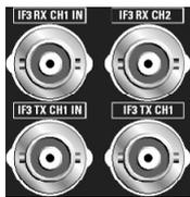
Four 50 Ω BNC connectors for option CMU-B17, I/Q and IF Interface:
