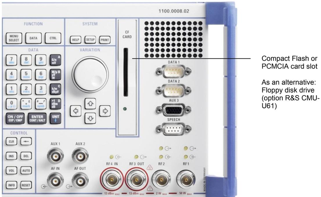
Fig. 1-7 CMU front view – Compact Flash card slot
